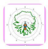
The picture illustrates the shielding effect of the rider when the antenna is placed in front of the motorcycle and shows how different antenna patterns are compared to cars. And the group will investigate the practical antenna performance for PTW in parallel.
