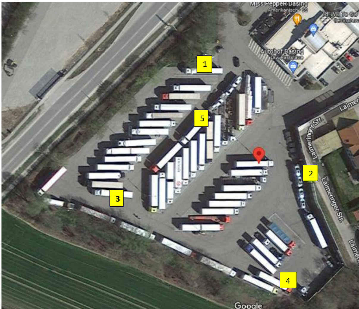
Figure 2: Example for truck blockings and limited paths at a truck parking site in Germany (Autohof Dasing A8)
