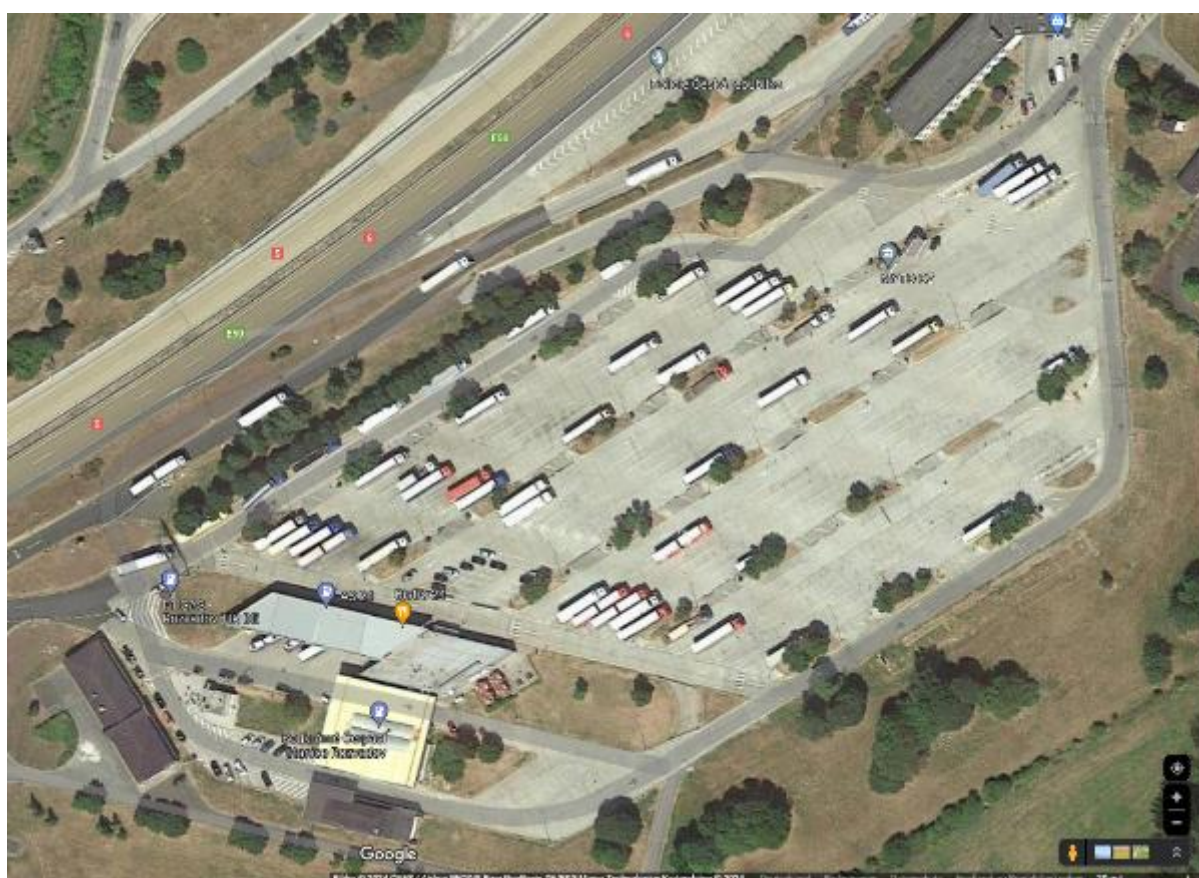
Figure 9: Example for a big parking site at the border to Germany with single access to the parking places which can easily be converted into a queue parking site.
