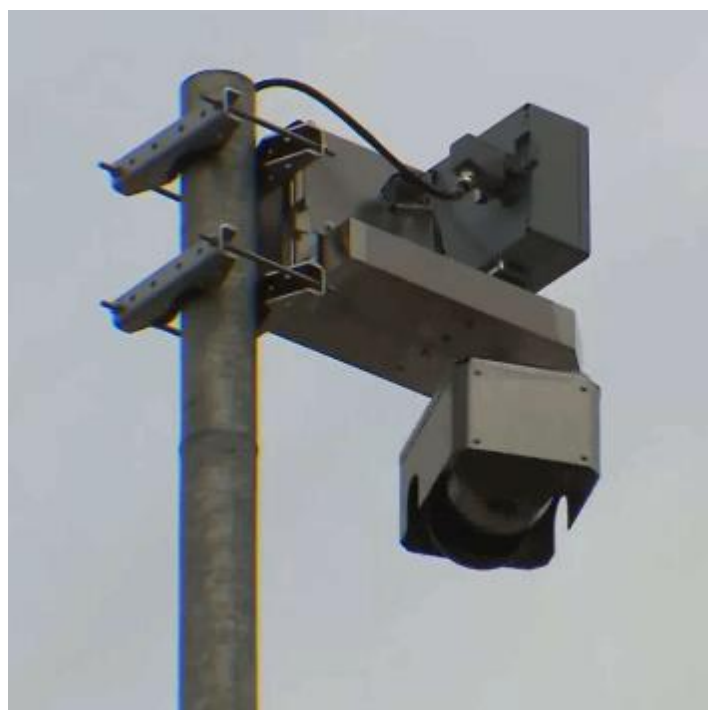
Figure 20: Detection of parking trucks by laser scanner
