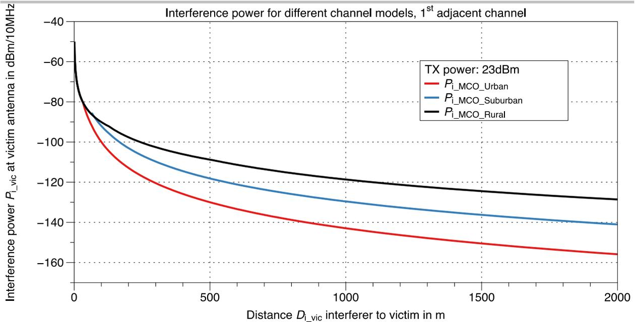
**Figure 12: Combined interference power  $P_{i\_vic}$  from 1<sup>st</sup> adjacent channel at victim antenna for the three channel models**
