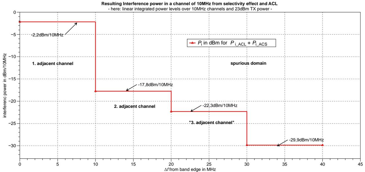
Figure 9: Effective interference power at the interfering TX  $P_{TX\_int\_eff}$  as combination of ACLR and ACS effect
