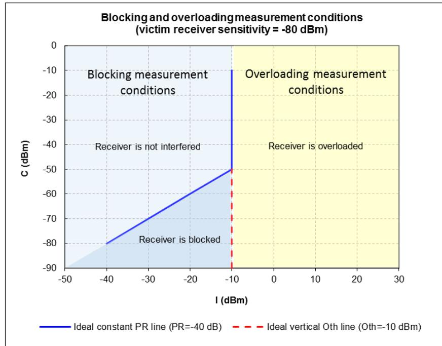
**Figure 10: Receiver blocking and overloading measurement ranges[ER-9]**
