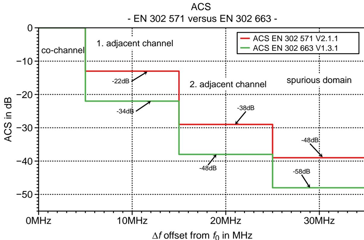
Figure 3: Adjacent channel selectivity ACS based on EN302 571 V2.1.1 [ER-3] and EN 302 663 V1.3.1, QPSK with  $R = \frac{1}{2}$  [ER-8]
