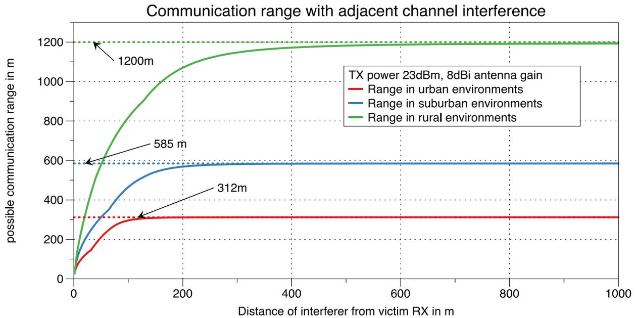
**Figure 15: Range reduction due to 1<sup>st</sup> adjacent channel interference for 23dBm TX power, extended range figure**
