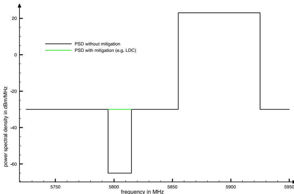
Figure 1: Regulatory spectrum mask in ECC Dec and Rec (08)01 in the year 2020 in dBm/MHz e.i.r.p.
