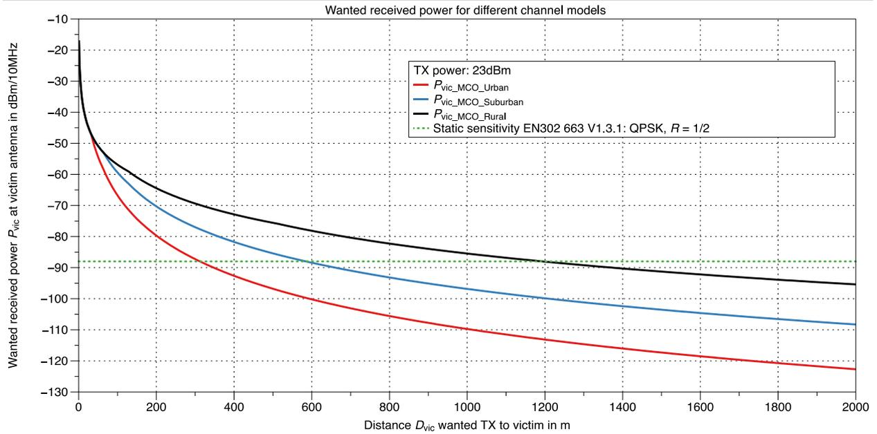
**Figure 13: Wanted link: Received power at victim antenna connector for different distances to wanted TX and different channel models including 8dBi antenna gain**
