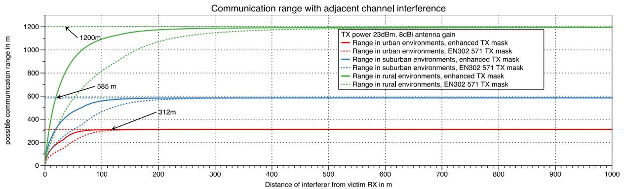
**Figure 19: Range Comparison of EN302 571 TX mask with optimized adjacent channel leakage interference mask**
