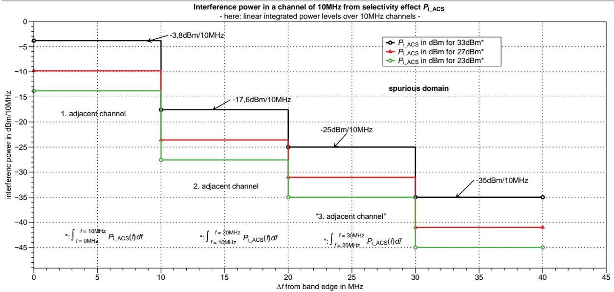
**Figure 4: Adjacent channel selectivity ACS: Interference power levels using linear integration**
