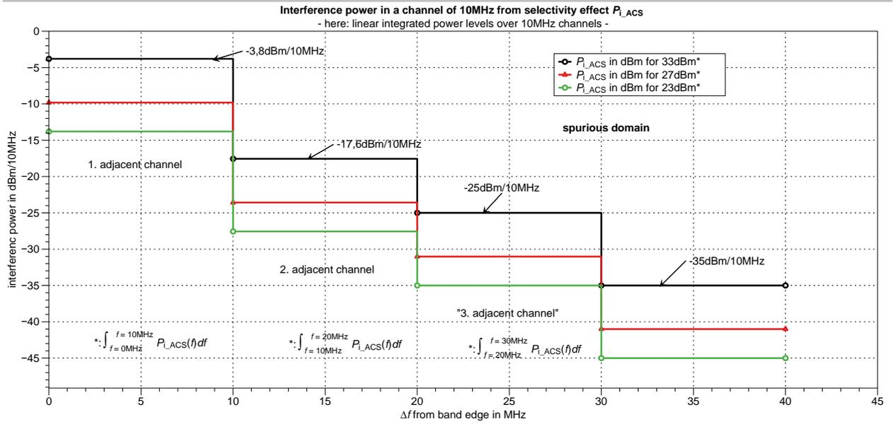
Figure 7: Effective interference levels  $P_{I\_ACS}$  from ACS effect for different TX power levels of the interfering transmitter.
