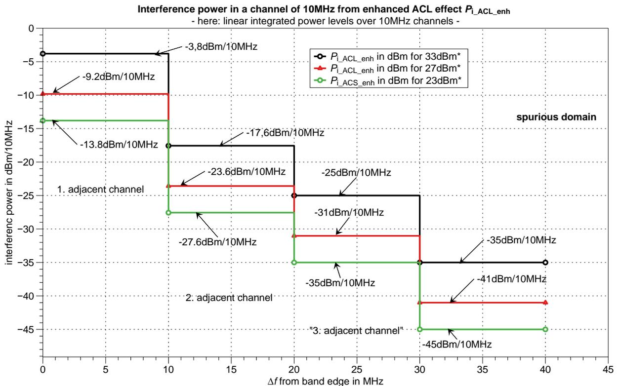
**Figure 18: optimized adjacent channel leakage interference power  $P_{i\_ACL\_enh}$  based on the ACS interference levels**
