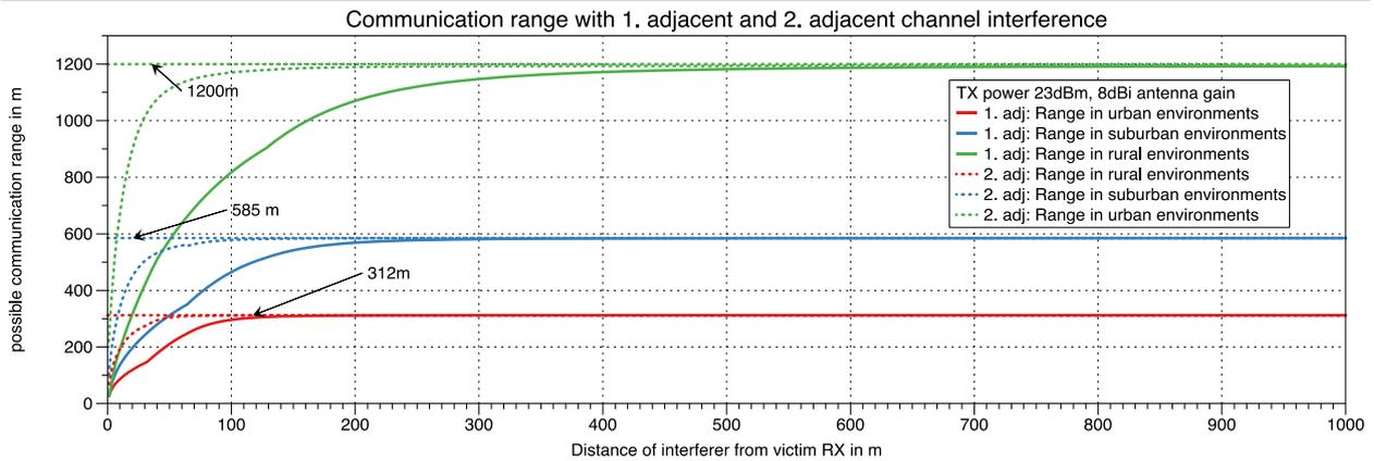
**Figure 17: Range reduction due to 1<sup>st</sup> adjacent and 2<sup>nd</sup> channel interference for 23dBm TX power, extended range figure**
