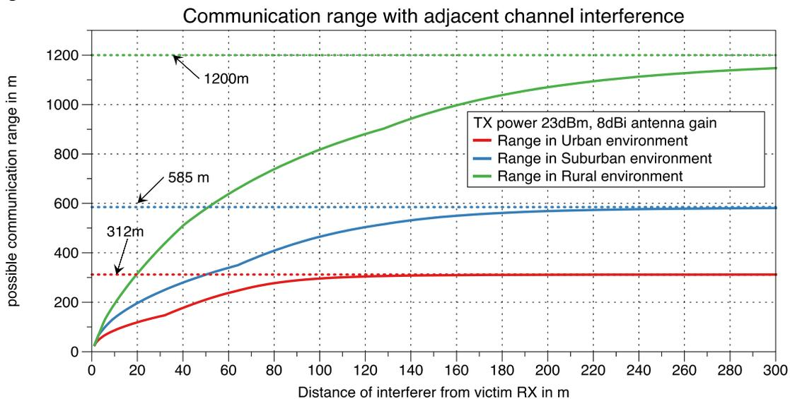
**Figure 14: Range reduction due to 1<sup>st</sup> adjacent channel interference for 23dBm TX power**
