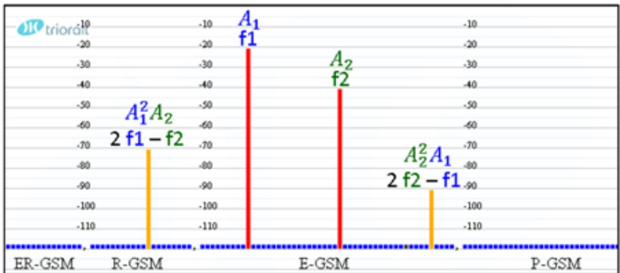
Figure 11: Generation of intermodulation products[ER-9]
