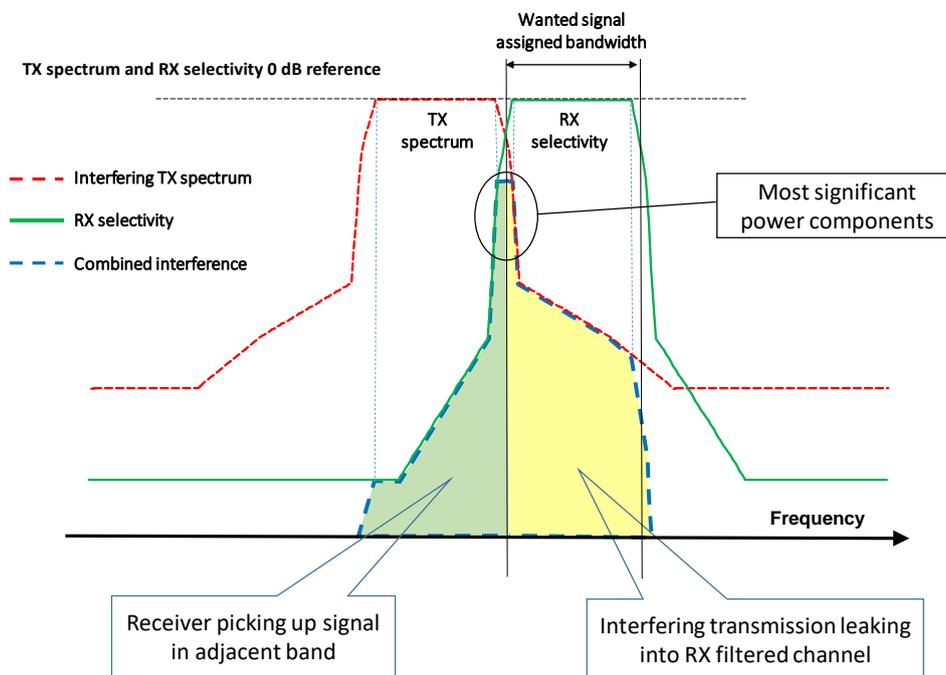
Figure 8: Impact of an interfering transmitter and a victim receiver on the reception of wanted signals, see ECC Report 310[ER-9]
