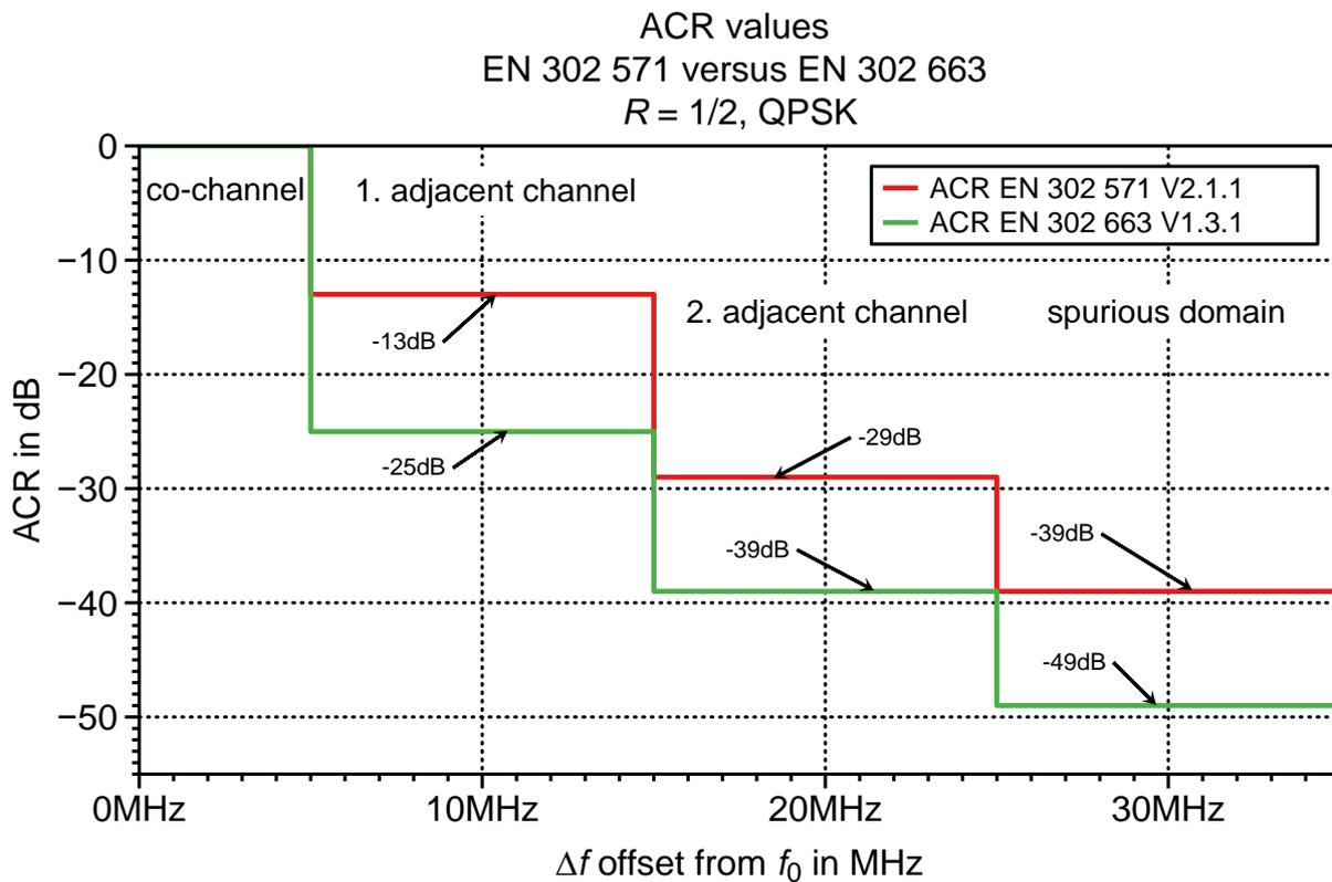
Figure 2: Adjacent channel rejection EN302 571 V2.1.1 [ER-3] and EN 302 663 V1.3.1, QPSK with R = 1/2 [ER-8]
