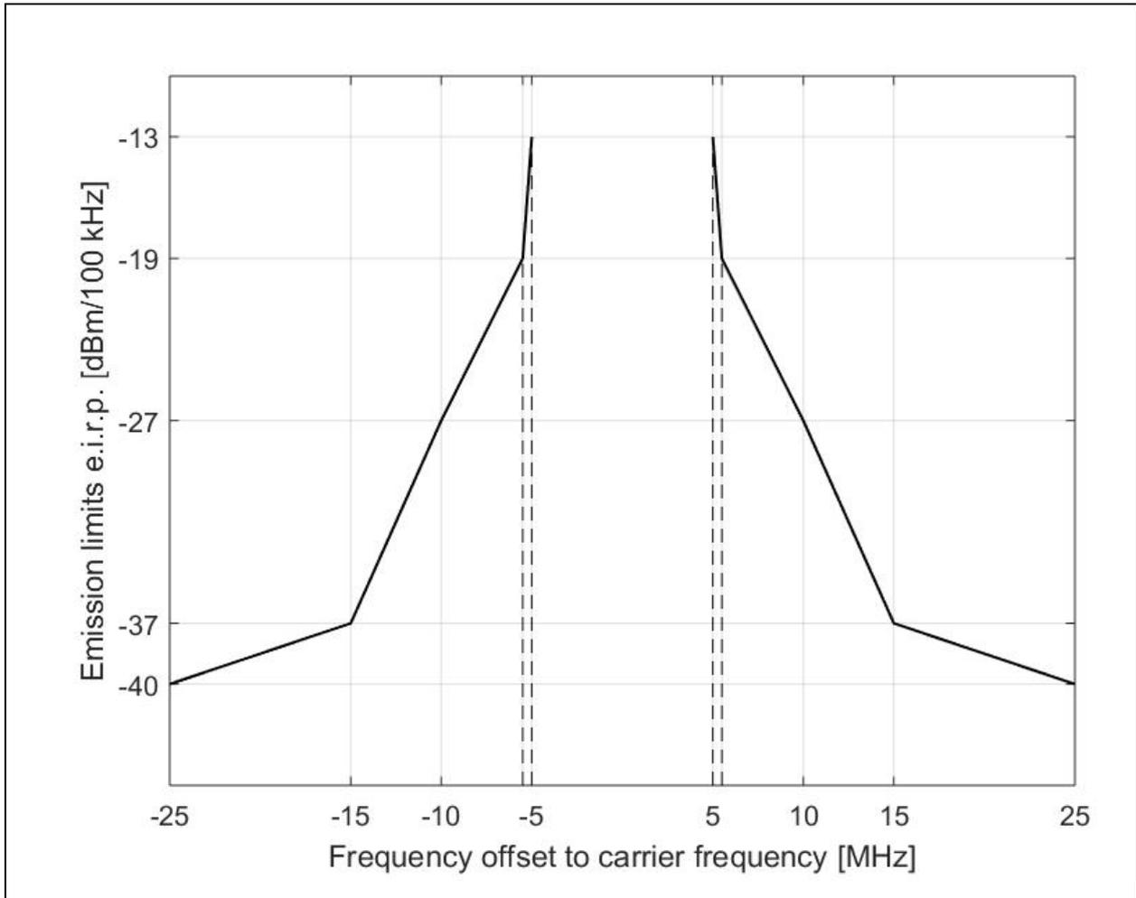
Figure 5: Transmitter spectrum mask EN 302 571 [ER-13]
