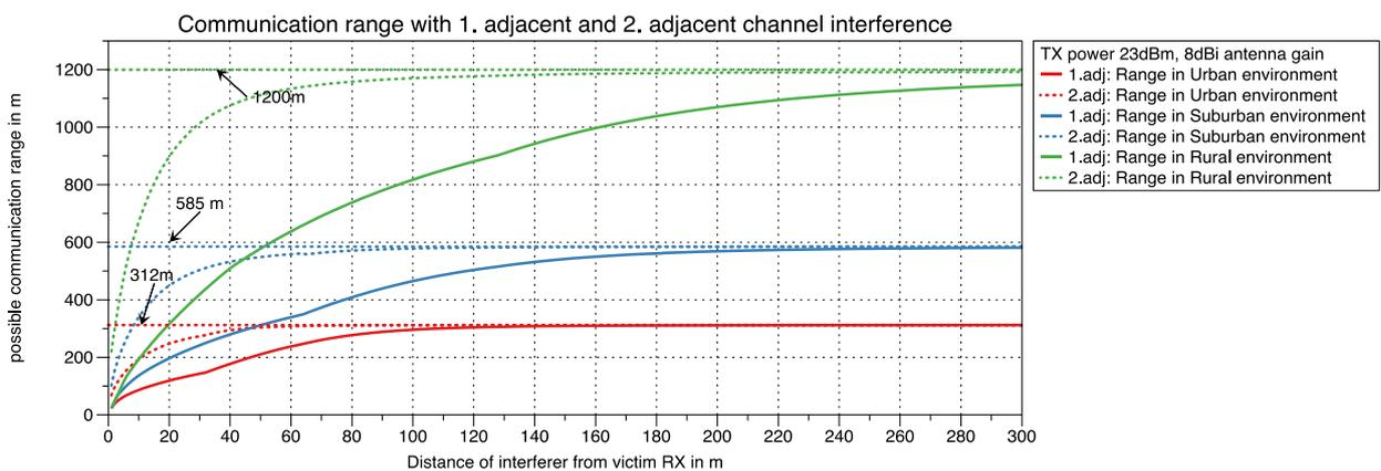
**Figure 16: Range reduction due to 1<sup>st</sup> and 2<sup>nd</sup> adjacent channel interference for 23dBm TX power**
