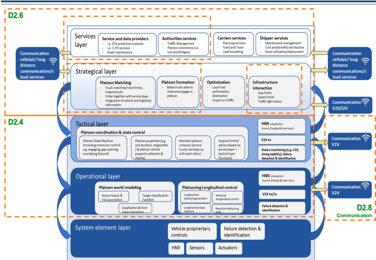
Figure 7: Layer Architecture for multi brand platooning (ENSEMBLE)
