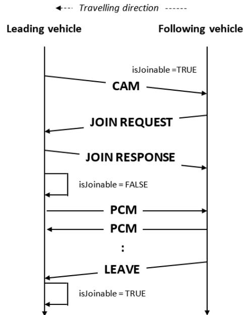
Figure 8: PCM information exchange example (ENSEMBLE)
