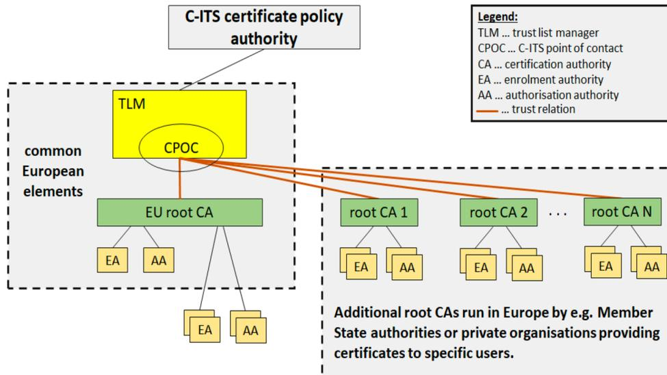
Figure 14: Certificate Trust Model Architecture
