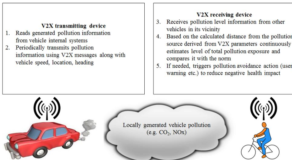
Figure 12: Simplified diagram of the V2X based emissions crowdsourcing approach
