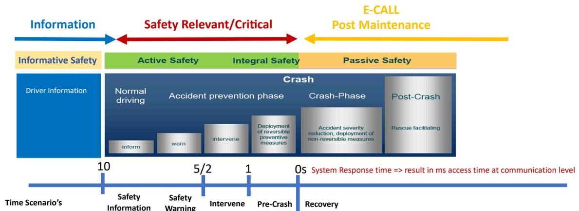
Figure 3: Phases of the vehicular safety system (Ref: C2C-CC)
