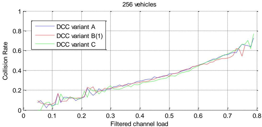
**Figure 5-71: Collision rate as a function of filtered channel load for 256 vehicles**
