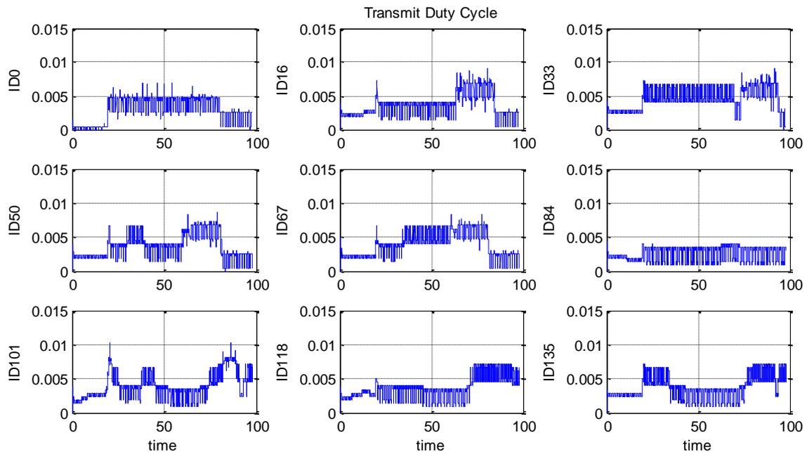
**Figure 5-92: Duty cycle for 9 selected vehicles, DCC variant C, 512 vehicles**
