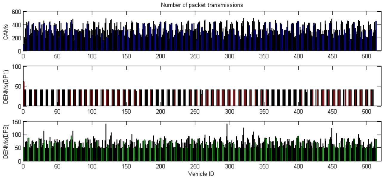
**Figure 5-85: Number of transmitted packets as a function of priority, modified DCC variant A, 512 vehicles**
