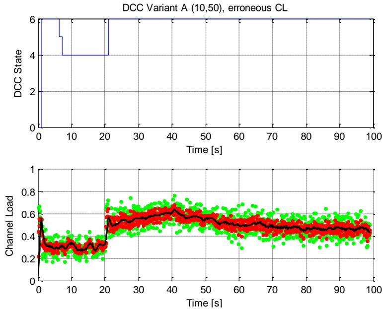
**Figure 5-74: DCC state adaptation and measured channel load of vehicle ID0 for DCC variant A with  $NDL\_TimeUp = 1s$ ,  $NDL\_TimeDown = 5s$ , 512 vehicles**
