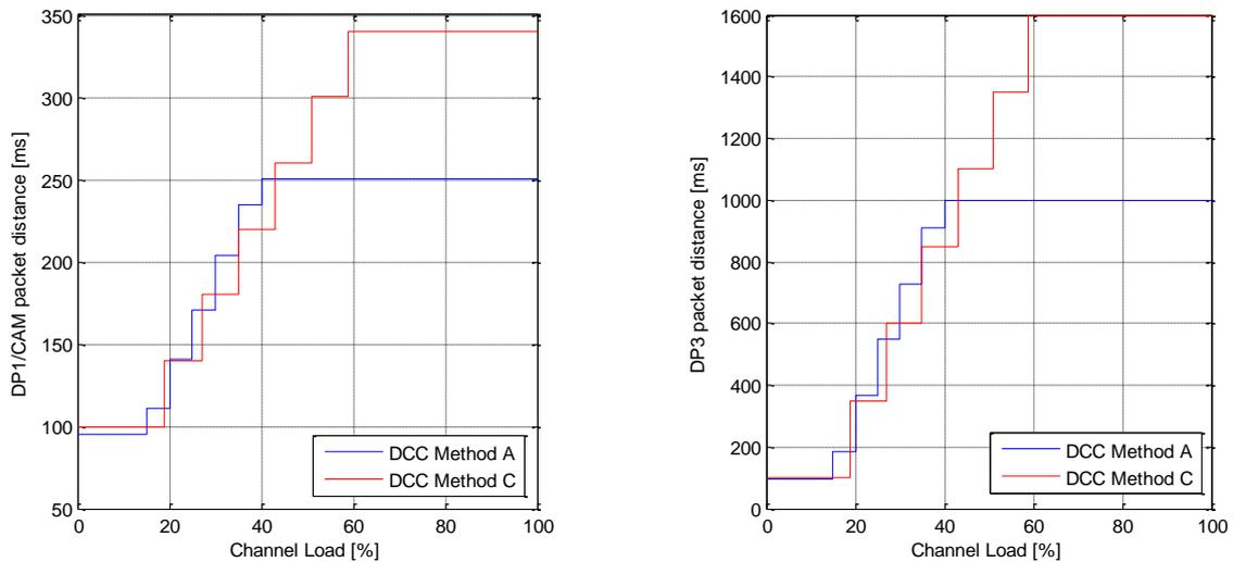
**Figure 3-5: Comparison of TOFF as a function of channel load of DCC Method A and C for DP1 and CAM packets (left) and DP3 packets (right)**
