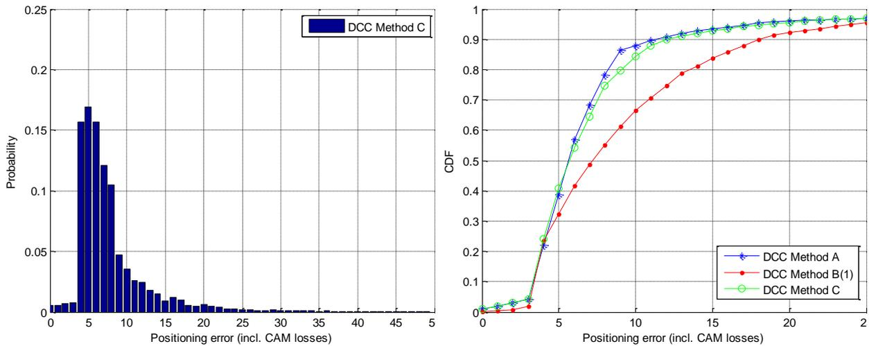
**Figure 5-70: Probability of position error for DCC variant C, 256 vehicles**
