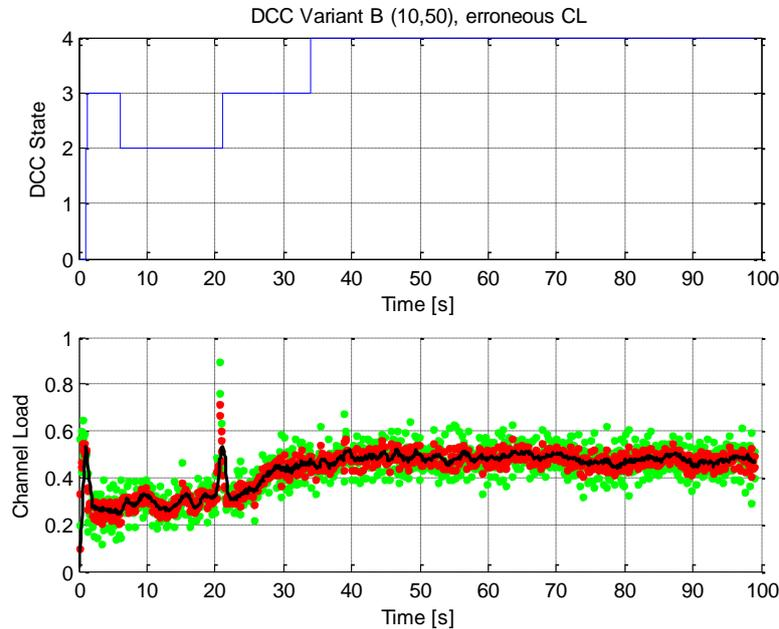
Figure 5-79: DCC state adaptation and measured channel load of vehicle ID0 for DCC variant B with  $NDL\_TimeUp = 1s$ .  $NDL\_TimeDown = 5s$ , 512 vehicles
