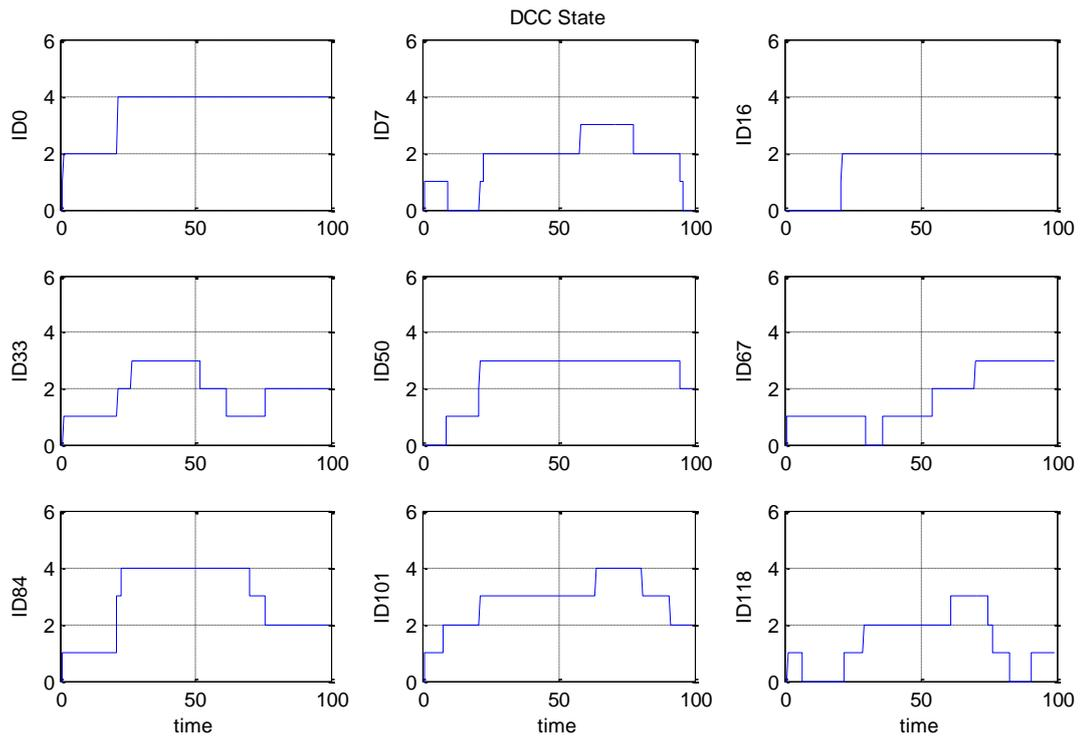
**Figure 5-30: DCC state for 9 selected vehicles, DCC variant C, 128 vehicles**
