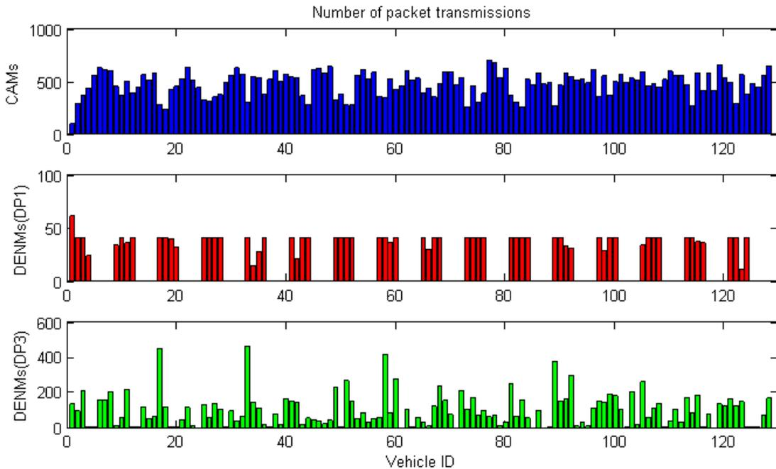
**Figure 5-18: Number of transmitted packets as a function of priority. DCC variant B, 128 vehicles**
