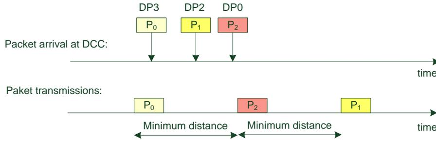
**Figure 3-3: Example for the transmission of packets in DCC variant B outside the DP0 burst mode**
