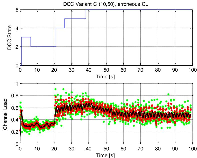
**Figure 5-84: DCC state adaptation and measured channel load of vehicle ID0 for modified DCC variant A with  $NDL\_TimeUp = 1s$ .  $NDL\_TimeDown = 5s$ , 512 vehicles**
