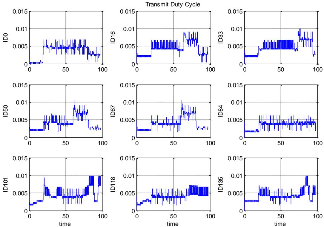
Figure 5-77: Duty cycle for 9 selected vehicles, DCC variant A, 512 vehicles
