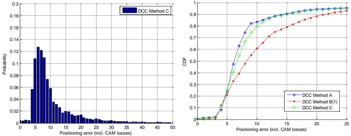
Figure 5-99: Probability of position error for DCC variant C and CDF, 512 vehicles
