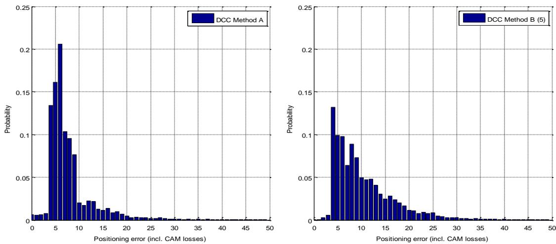
**Figure 5-68: Probability of position error for DCC variant A (left) and DCC variant B with a CAM queue length of 5 (right) based on received CAM packets, 256 vehicles**
