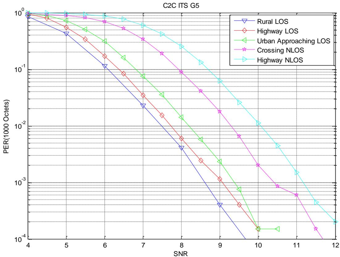
**Figure 3-6: Packet error rate for 6Mbps and 1000 Octets**
