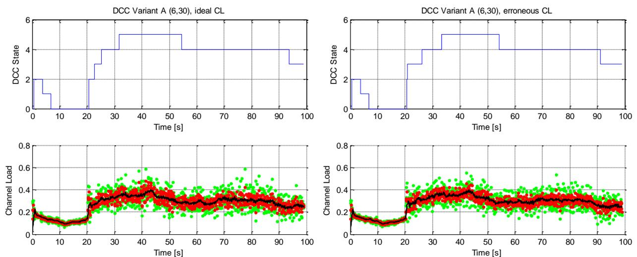
**Figure 5-6: DCC state adaptation and measured channel load of vehicle ID2 for DCC variant A with *NDL\_TimeUp* =0.6s, *NDL\_TimeDown* =3s**
