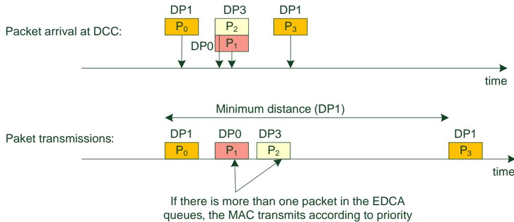
**Figure 3-2: Example for the transmission of packets in DCC variant A**
