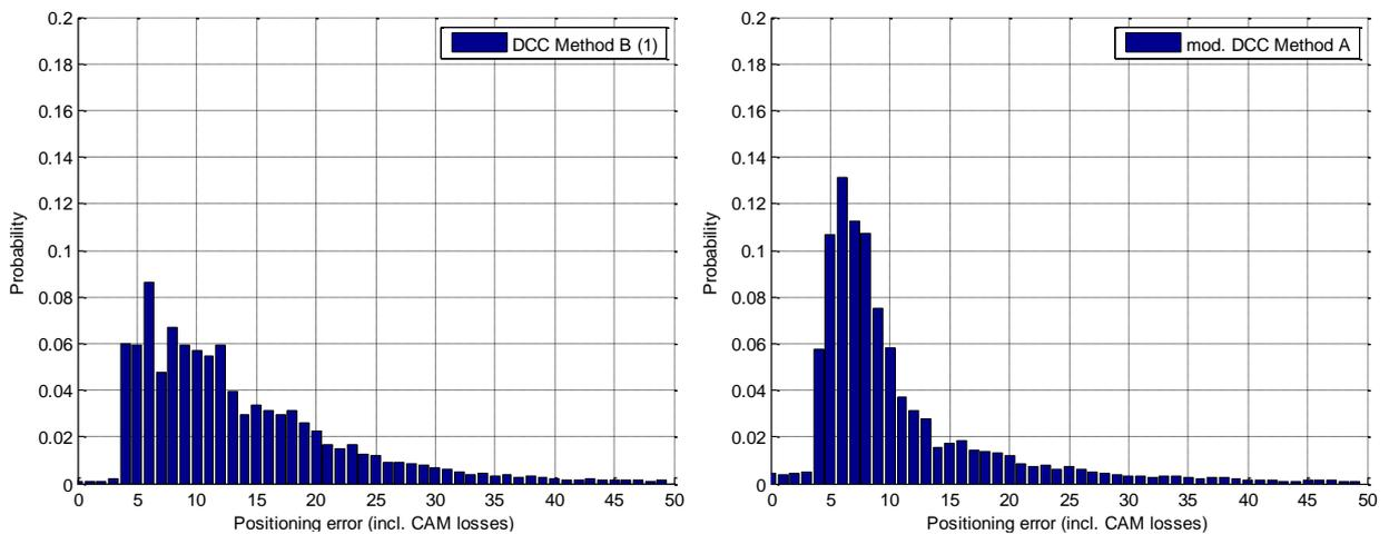
**Figure 5-98: Probability of position error for DCC variant B with a CAM queue length of 1 (left) and modified DCC variant A (right) based on received CAM packets, 512 vehicles**
