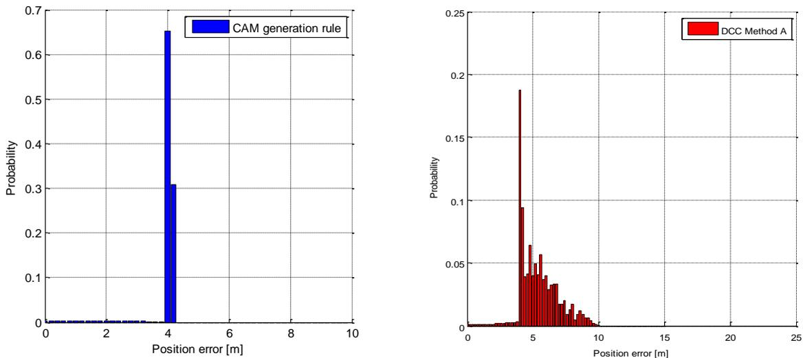
**Figure 5-33: Probability of position error using CAM generation rule and no DCC limitations (left) and DCC variant A (right), 128 vehicles**
