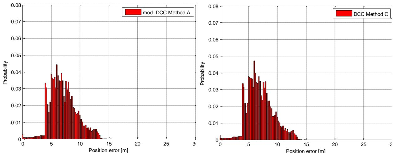
**Figure 5-96: Probability of position error for modified DCC variant A (left) and DCC variant C (right) based on transmitted CAM packets**
