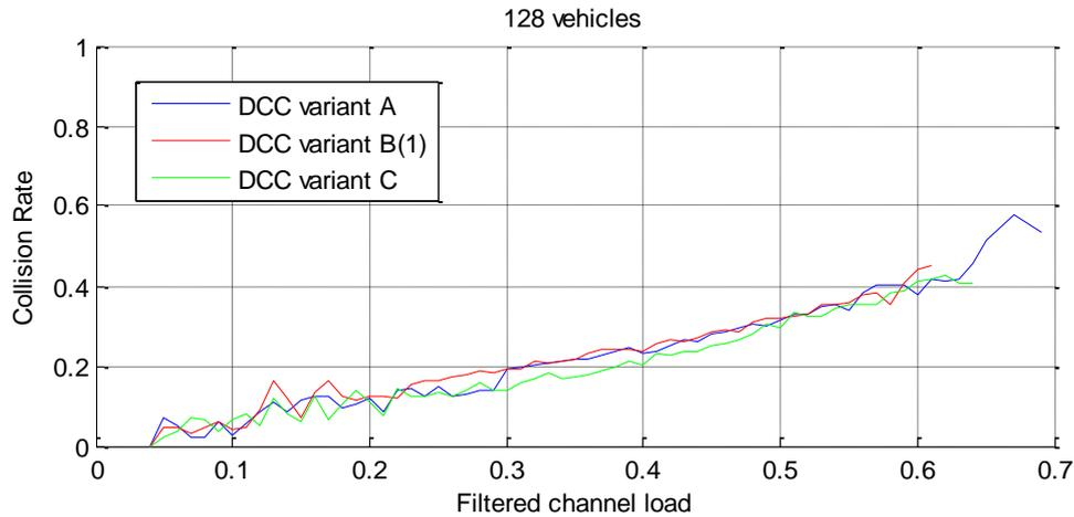
**Figure 5-40: Collision rate as a function of filtered channel load for 128 vehicles, post-crash**
