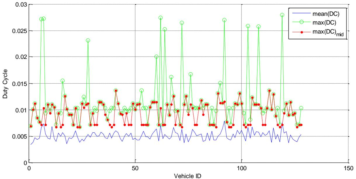
**Figure 5-27: Mean and maximum duty cycle, modified DCC variant A, 128 vehicles**
