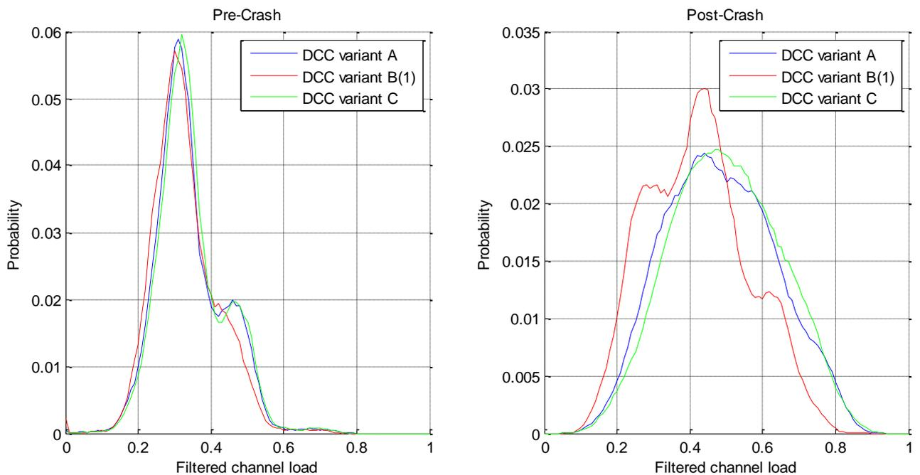
**Figure 5-101: Probability function of the filtered channel load during pre-crash and post-crash phase, 512 vehicles**
