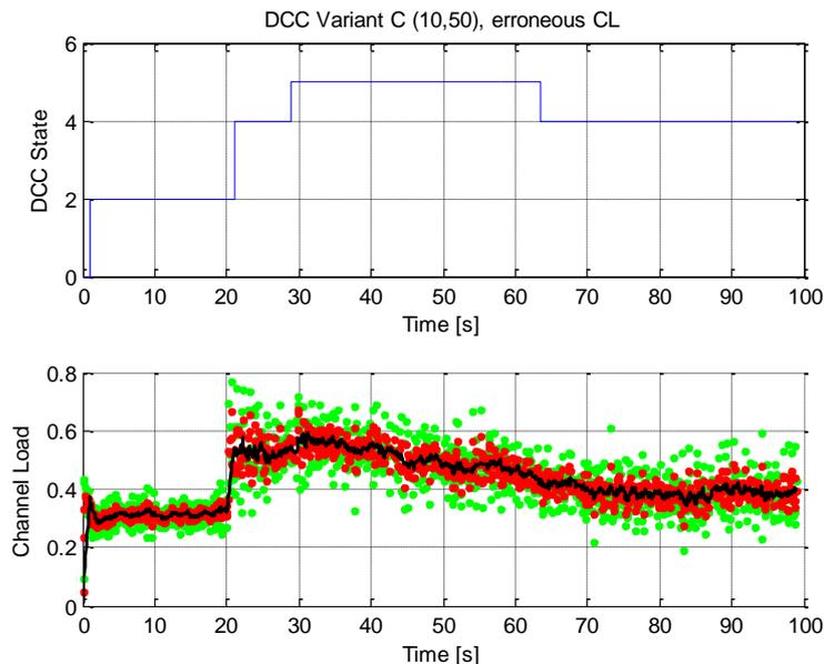
**Figure 5-28: DCC state adaptation and measured channel load of vehicle ID2 for DCC variant C with  $NDL\_TimeUp = 1s$ ,  $NDL\_TimeDown = 5s$ , 128 vehicles**
