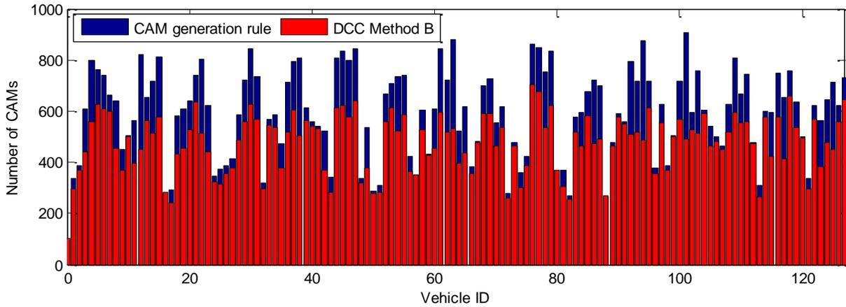
**Figure 5-19: Number of CAMs according to CAM generation rule (blue) and at the input of the DCC (red), DCC variant B, 128 vehicles**
