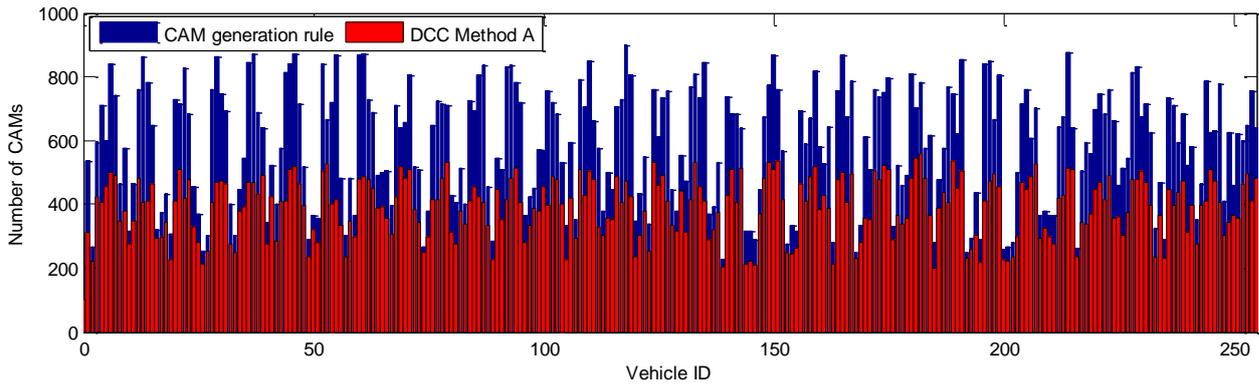
**Figure 5-45: Number of CAMs according to CAM generation rule (blue) and at the input of the DCC (red), DCC variant A, 256 vehicles**
