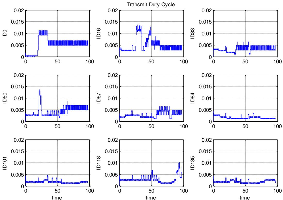
**Figure 5-53: Duty cycle for 9 selected vehicles, DCC variant B, 256 vehicles**
