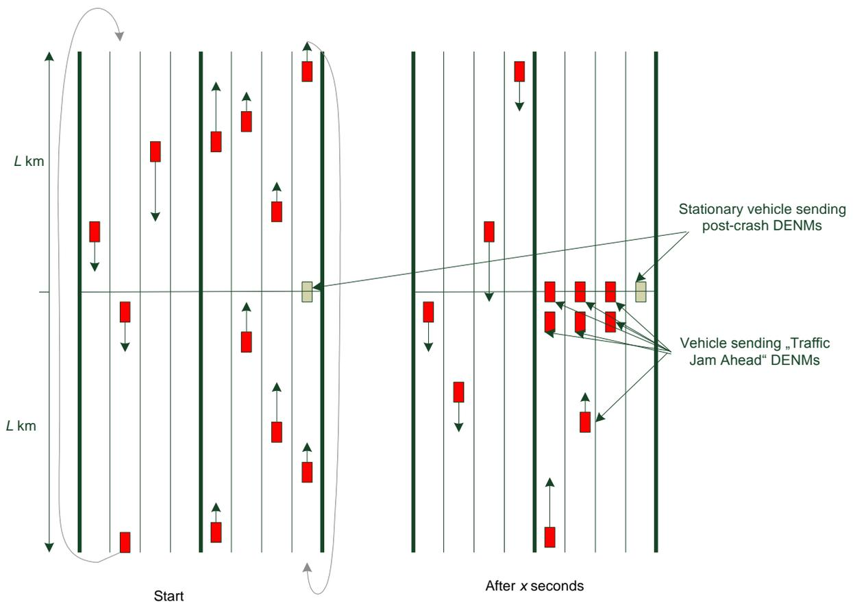
Figure 5-1: Scenario (Highway with accident and traffic jam)
