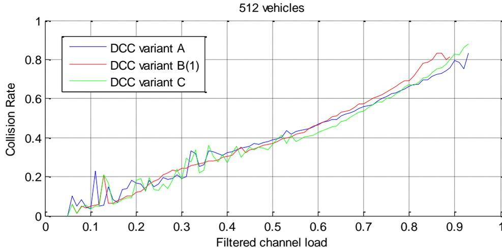
**Figure 5-100: Collision rate as a function of filtered channel load for 512 vehicles**
