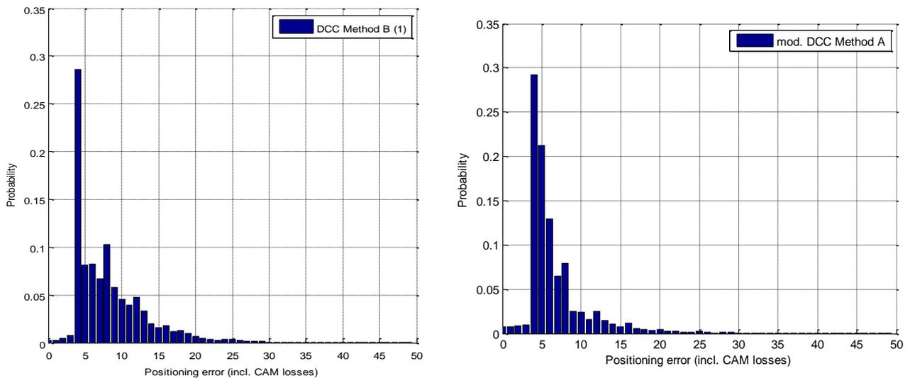
**Figure 5-38: Probability of position error for DCC variant B with a CAM queue length of 1 (left) and the modified DCC variant A (right) based on received CAM packets, 128 vehicles**
