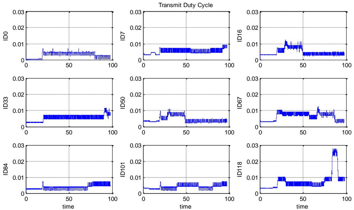
**Figure 5-26: Duty cycle for 9 selected vehicles, modified DCC variant A, 128 vehicles**
