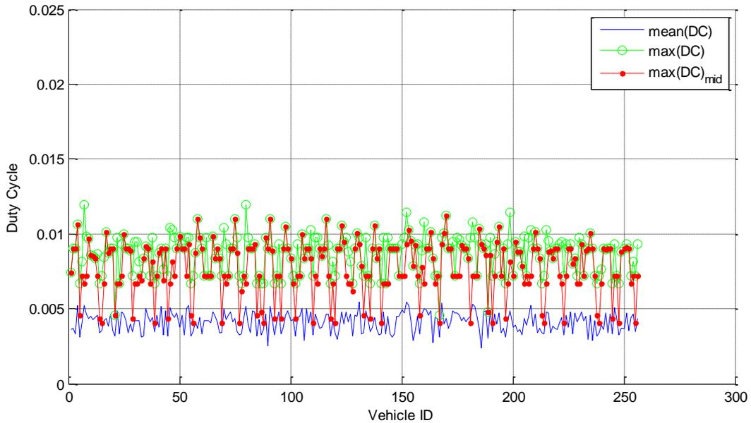
Figure 5-64: Mean and maximum duty cycle, DCC variant C, 256 vehicles
