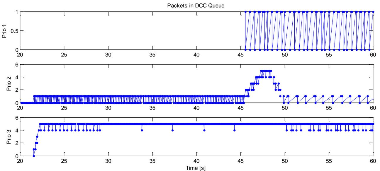
**Figure 5-17: Priority dependent number of packets in the DCC buffer for vehicle ID2 in the highway scenario with 128 vehicles**
