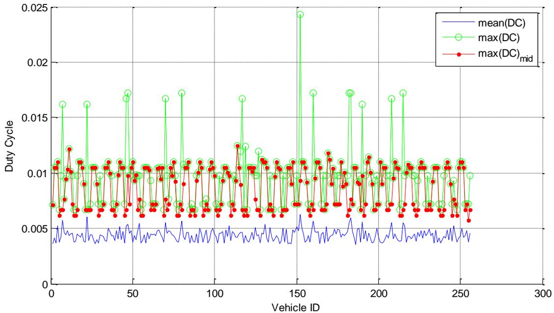
**Figure 5-48: Mean and maximum duty cycle, DCC variant A, 256 vehicles**
