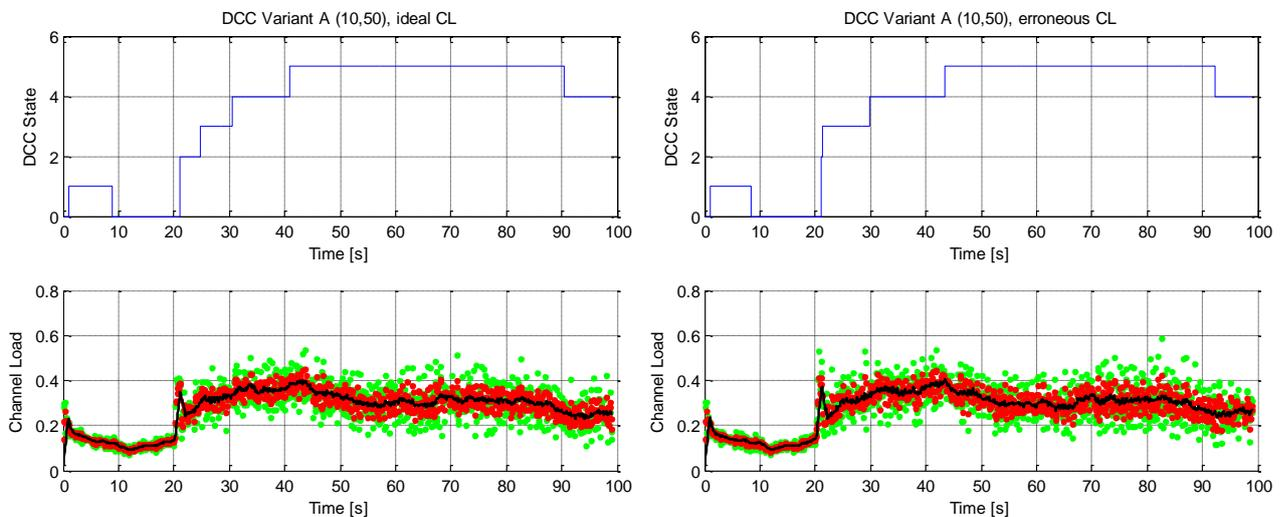
Figure 5-5: DCC state adaptation and measured channel load of vehicle ID2 for DCC variant A with *NDL\_TimeUp* =1s, *NDL\_TimeDown* =5s
