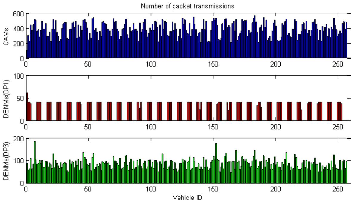
**Figure 5-56: Number of transmitted packets as a function of priority, modified DCC variant A, 256 vehicles**
