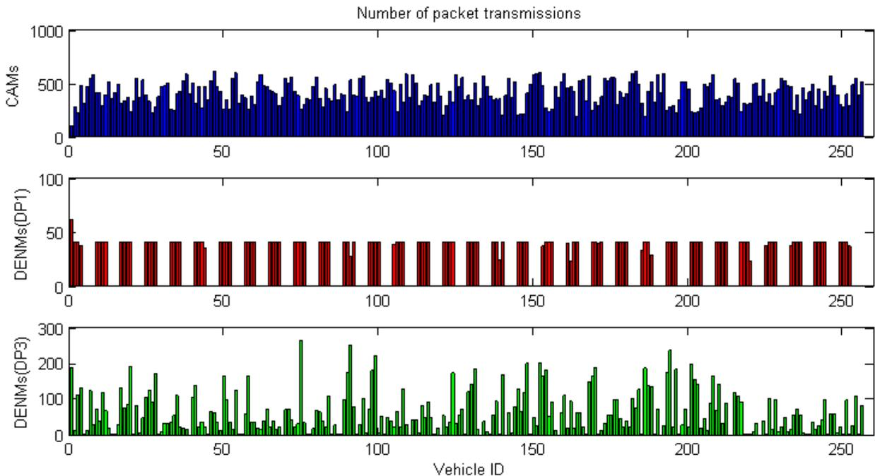
**Figure 5-50: Number of transmitted packets as a function of priority, DCC variant B, 256 vehicles**
