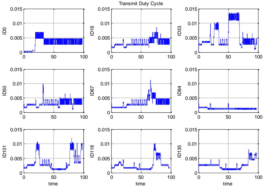
**Figure 5-82: Duty cycle for 9 selected vehicles, DCC variant B, 512 vehicles**
