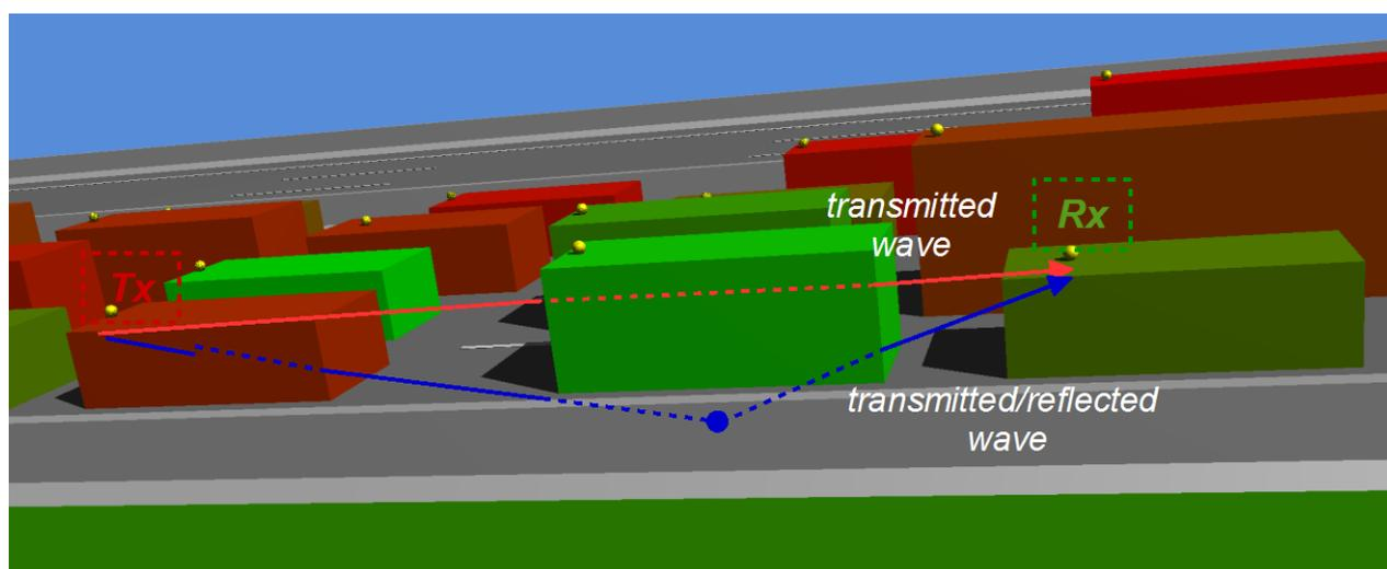
Figure 4-3: Obstructed line-of-sight scenario: direct path ray transmitted (through obstructing vehicle between Tx and Rx) and a ground reflected ray. Yellow spheres mark antenna positions.
