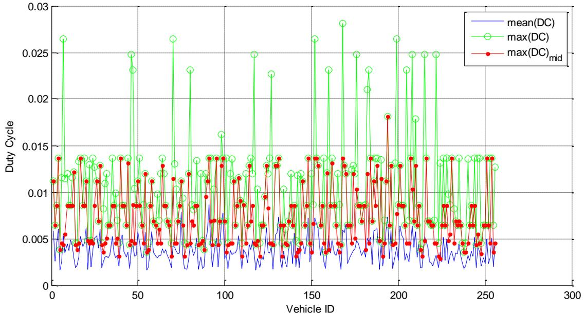
Figure 5-54: Mean and maximum duty cycle, DCC variant B, 256 vehicles
