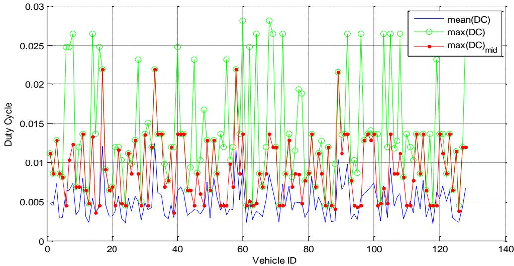
**Figure 5-22: Mean and maximum duty cycle, DCC variant B, 128 vehicles**
