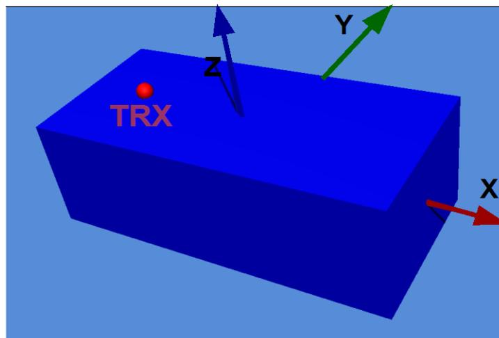
Figure 4-2: Simplified box-car-model for VW-Scirocco (L x W x H) = (4.25 x 2.0 x 1.4) m.
