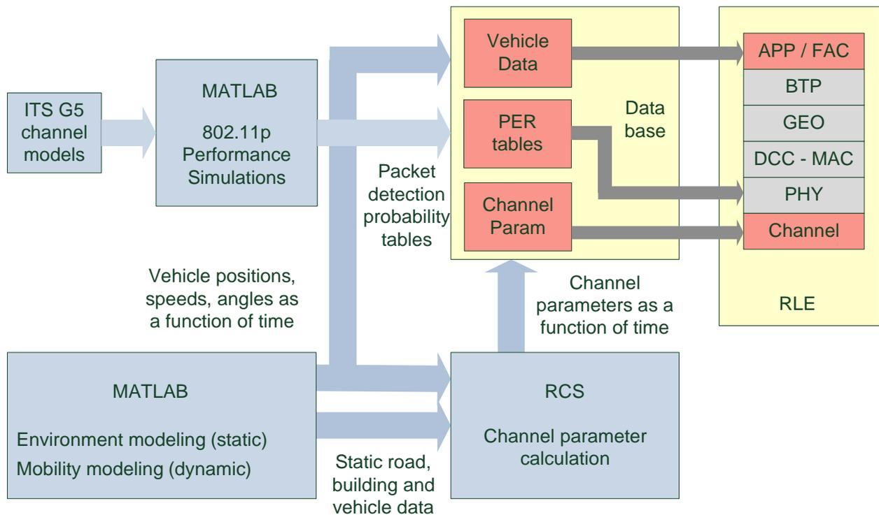
**Figure 2-1: IMST framework for C2C simulations**
