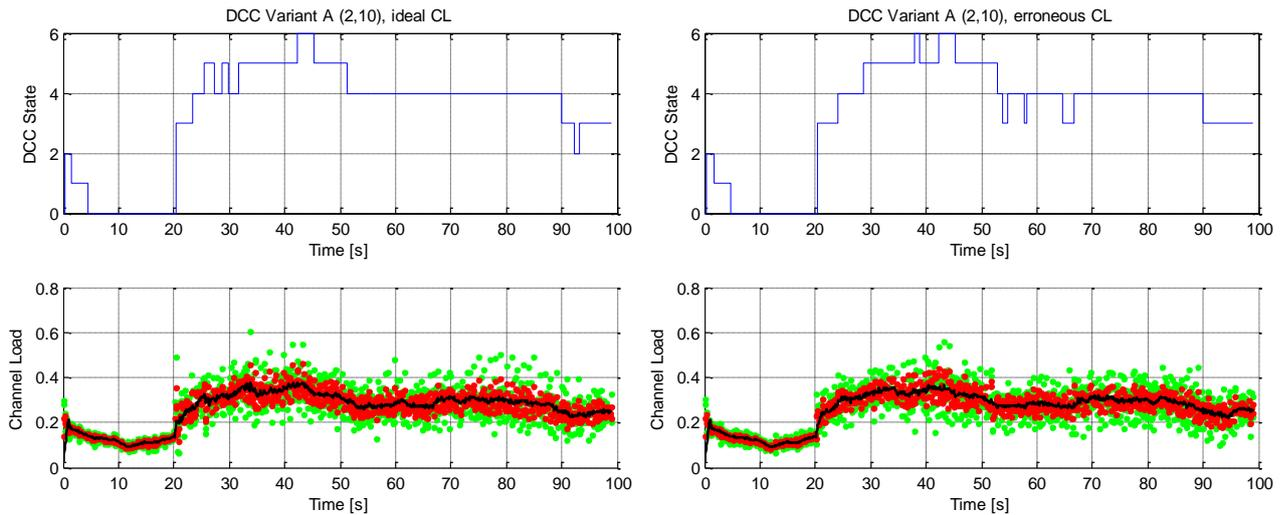
**Figure 5-7: DCC state adaptation and measured channel load of vehicle ID2 for DCC variant A with  $NDL\_TimeUp = 0.2s$ ,  $NDL\_TimeDown = 1.0s$**
