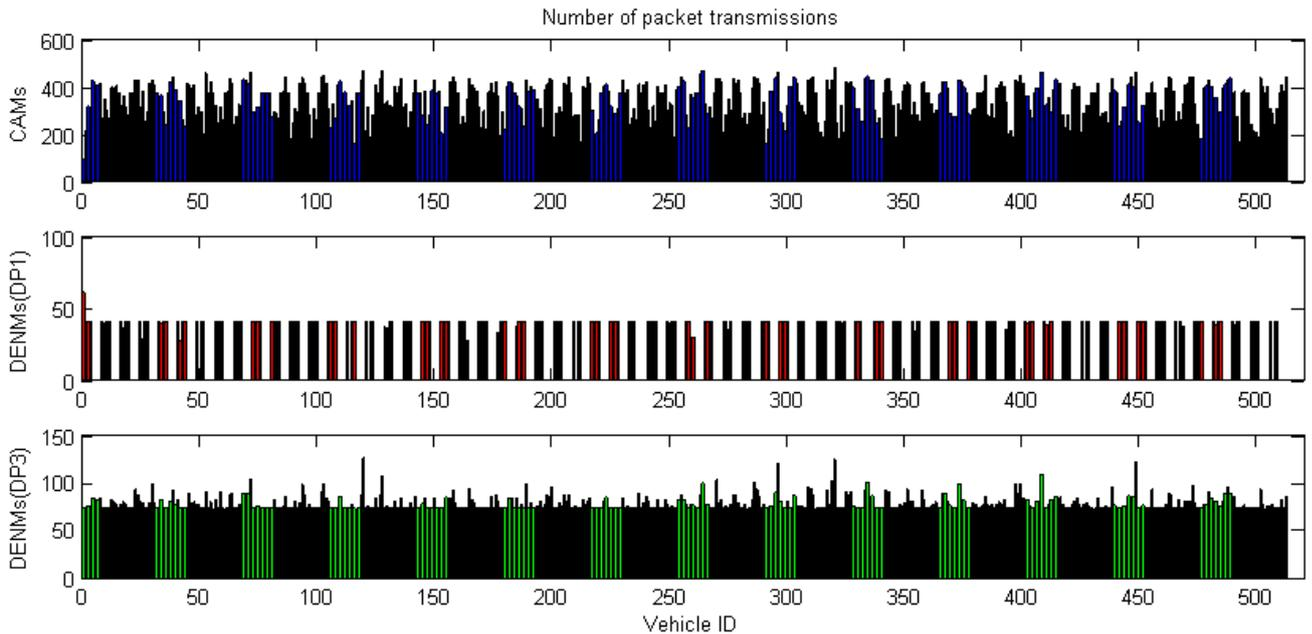
**Figure 5-75: Number of transmitted packets as a function of priority, DCC variant A, 512 vehicles**
