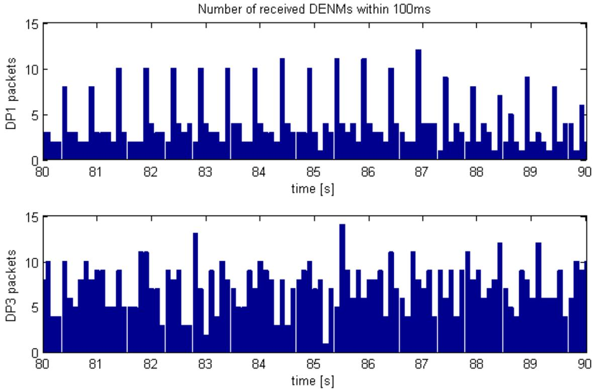
Figure 5-4: Periodicity of the number received DP1 and DP3 of vehicle ID2
