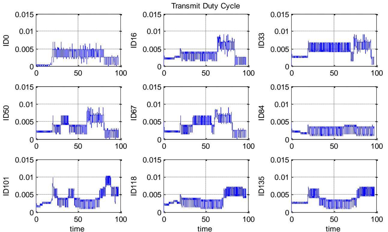
Figure 5-87: Duty cycle for 9 selected vehicles, modified DCC variant A, 512 vehicles
