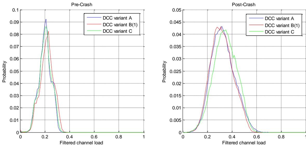
**Figure 5-41: Probability function of the filtered channel load during pre-crash and post-crash phase, 128 vehicles**
