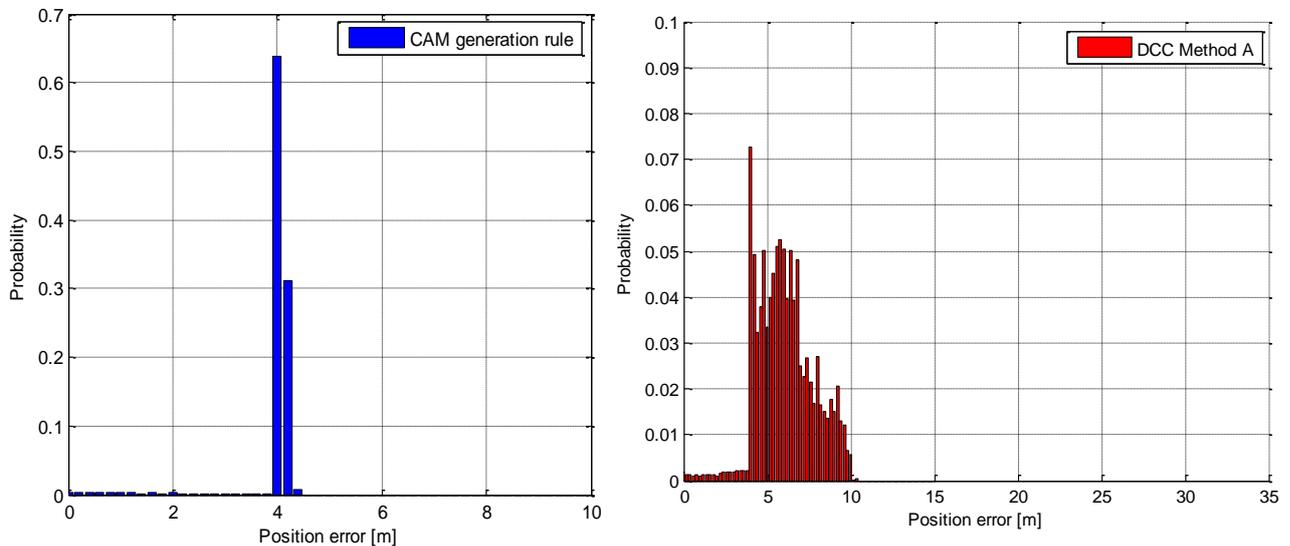
Figure 5-65: Probability of position error for using CAM generation rule and no DCC limitations (left) and DCC variant A (right) based on transmitted CAM packets, 256 vehicles
