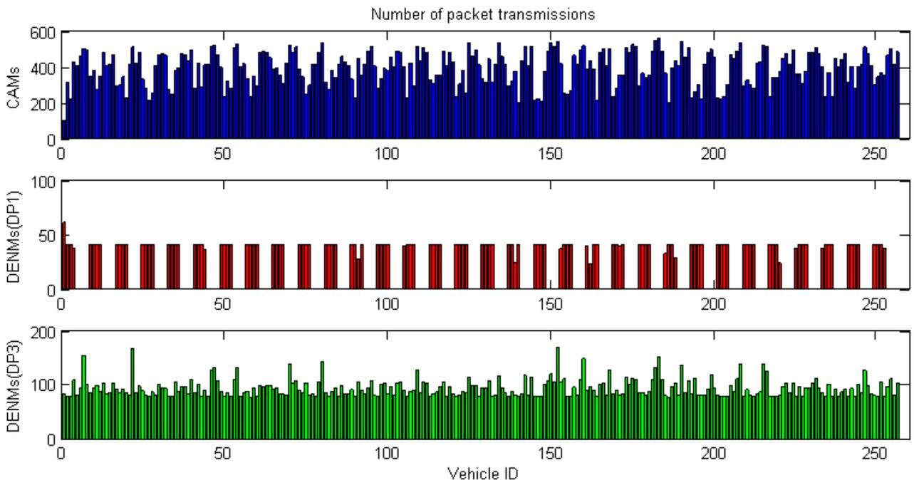
**Figure 5-44: Number of transmitted packets as a function of priority, DCC variant A, 256 vehicles**
