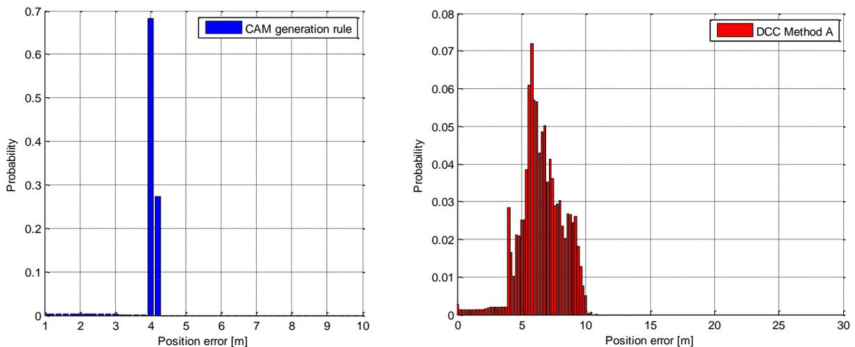
Figure 5-94: Probability of position error for using CAM generation rule and no DCC limitations (left) and DCC variant A (right) based on transmitted CAM packets
