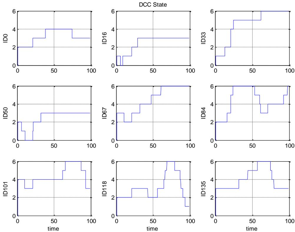
Figure 5-62: DCC State for 9 selected vehicles, DCC variant C, 256 vehicles
