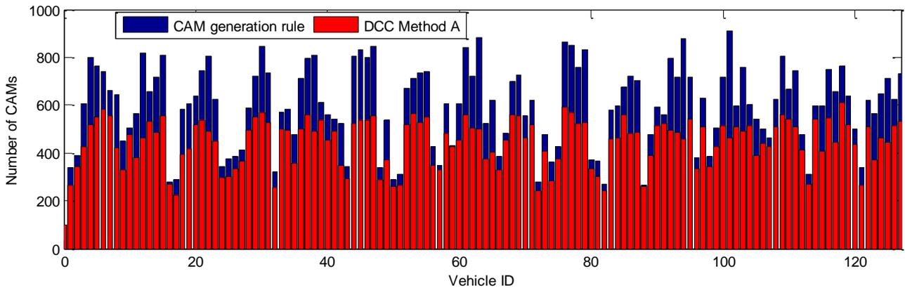
**Figure 5-11: Number of CAMs according to CAM generation rule (blue) and at the input of the DCC (red), DCC variant A, 128 vehicles**
