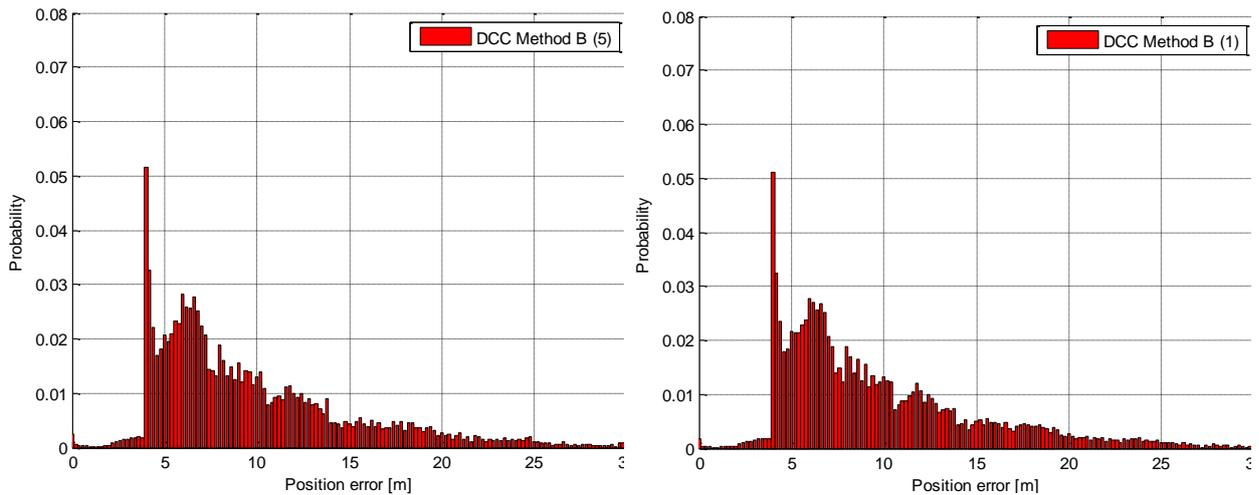
**Figure 5-95: Probability of position error for DCC variant B with a CAM queue length of 5 (left) and 1 packet (right) based on transmitted CAM packets**
