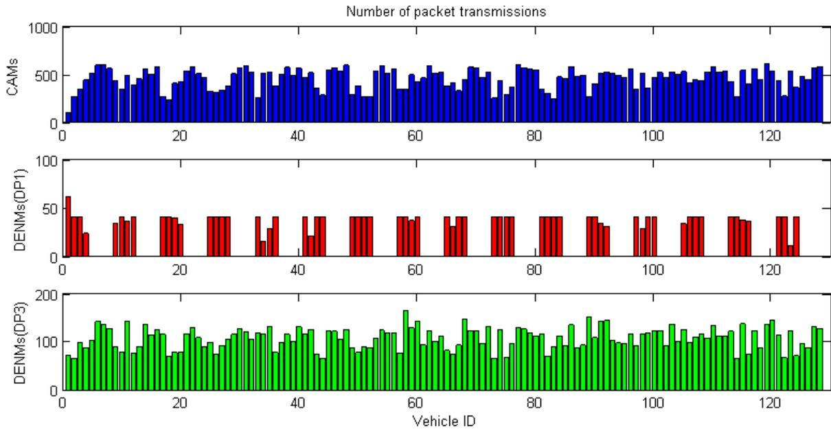
**Figure 5-29: Number of transmitted packets as a function of priority. DCC variant C, 128 vehicles**
