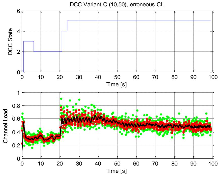
Figure 5-89: DCC state adaptation and measured channel load of vehicle ID0 for DCC variant C with  $NDL\_TimeUp = 1s$ ,  $NDL\_TimeDown = 5s$ , 512 vehicles
