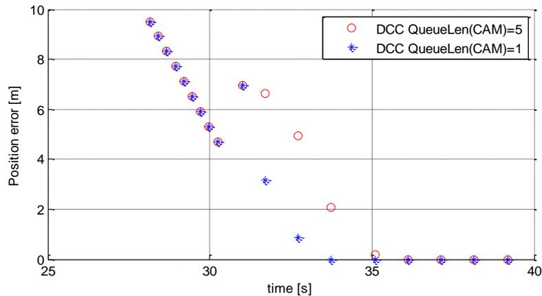
**Figure 5-35: Resulting position error for a DCC queue length of 5 (red) and 1 packet (blue)**
