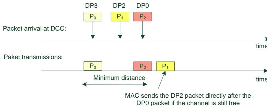
**Figure 3-4: Example for the transmission of packets in DCC variant B inside the DP0 burst mode**
