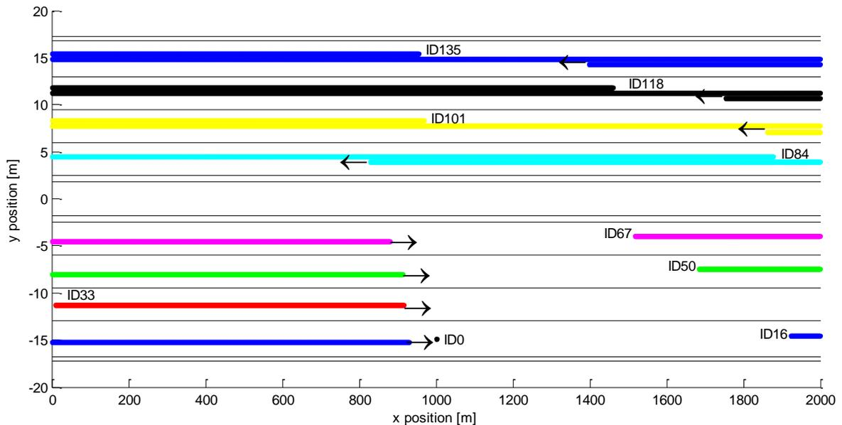
**Figure 5-42: Traces of 9 selected vehicles, highway scenario with 256 vehicles**
