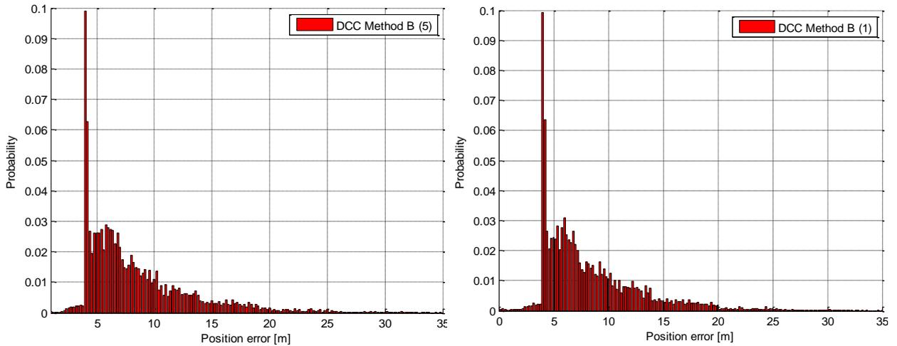
**Figure 5-66: Probability of position error for DCC variant B with a CAM queue length of 5 (left) 1 packet (right) based on transmitted CAM packets, 256 vehicles**
