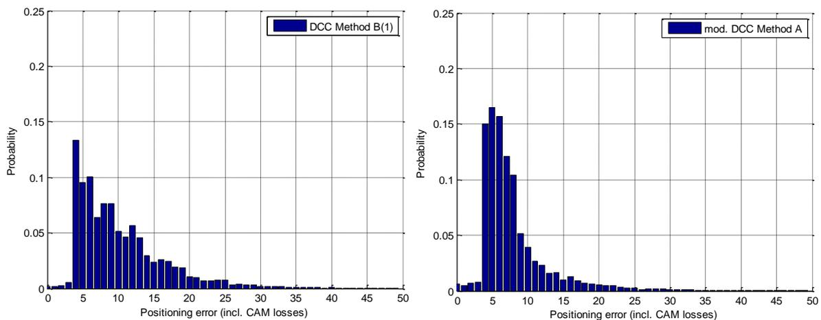
**Figure 5-69: Probability of position error for DCC variant B with a CAM queue length of 1 (left) and the modified DCC variant A (right) based on received CAM packets, 256 vehicles**
