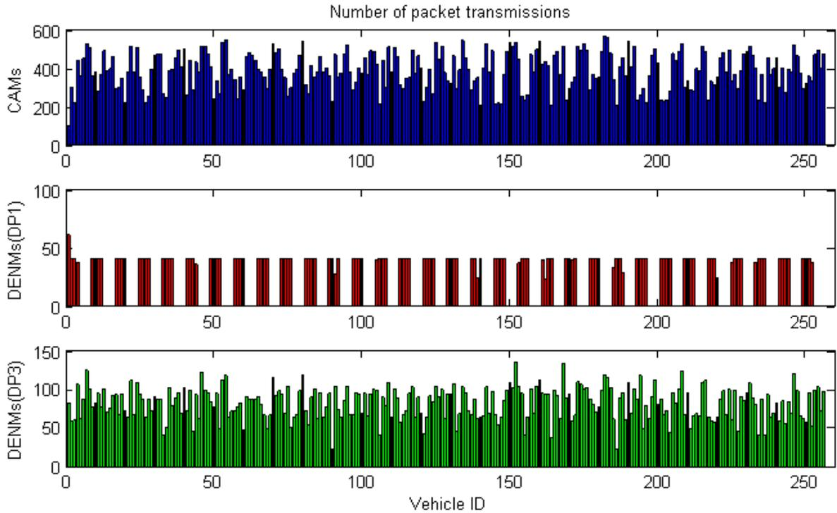
Figure 5-61: Number of transmitted packets as a function of priority, DCC variant C, 256 vehicles
