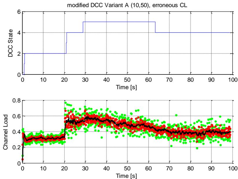
Figure 5-55: DCC state adaptation and measured channel load of vehicle ID2 for modified DCC variant A with  $NDL\_TimeUp = 1s$ ,  $NDL\_TimeDown = 5s$ , 256 vehicles
