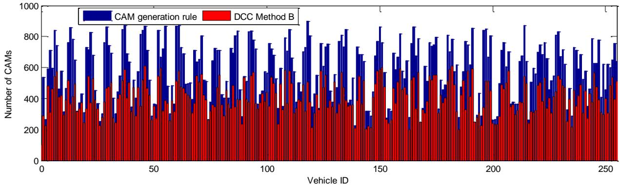
**Figure 5-51: Number of CAMs according to CAM generation rule (blue) and at the input of the DCC (red), DCC variant B, 256 vehicles**
