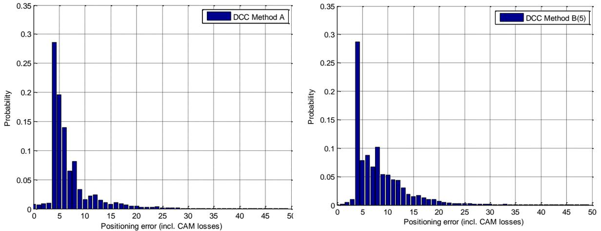
**Figure 5-37: Probability of position error for DCC variant A (left) and DCC variant B (right) with a CAM queue length of 5 packets based on CAM packet receptions, 128 vehicles**
