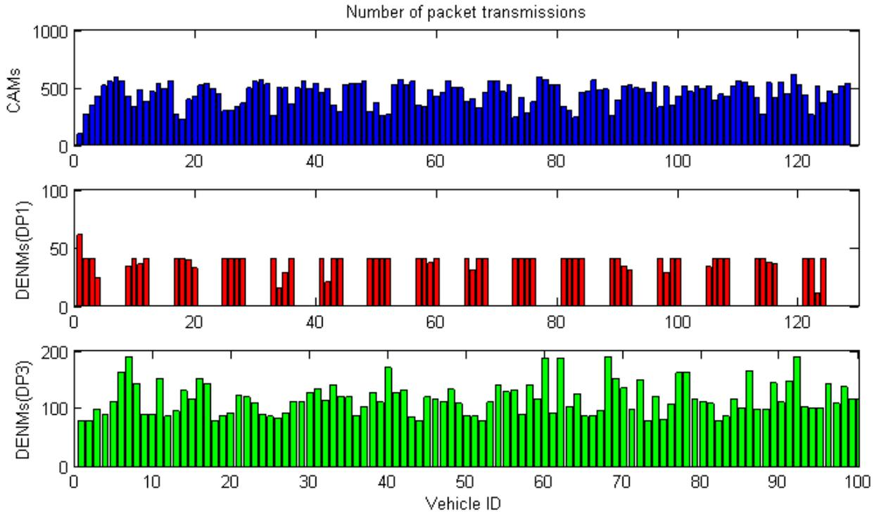
Figure 5-8: Number of transmitted packets as a function of priority, DCC variant A, 128 vehicles
