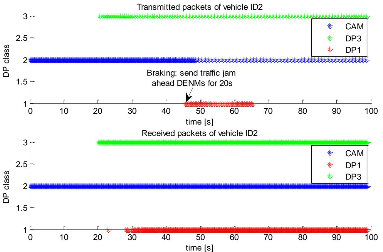
**Figure 5-3: Transmitted and received DP1, CAM and DP3 packets of vehicle ID2**
