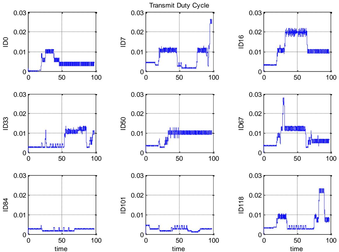
Figure 5-21: Duty cycle for 9 selected vehicles, DCC variant B, 128 vehicles
