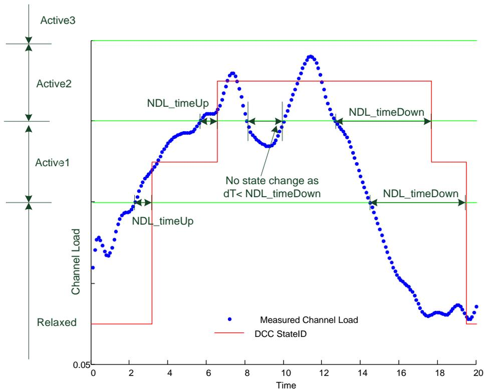
**Figure 3-1: DCC state as a function of the measured channel load**
