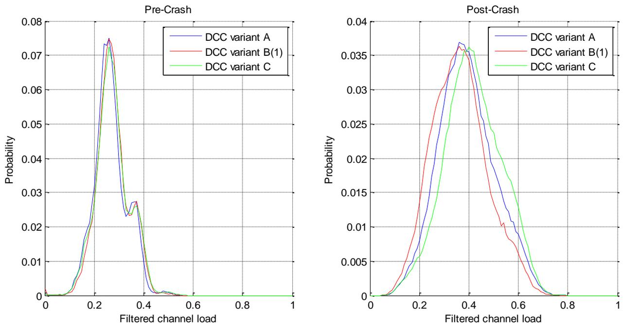
**Figure 5-72: Probability function of the filtered channel load during pre-crash and post-crash phase, 256 vehicles**
