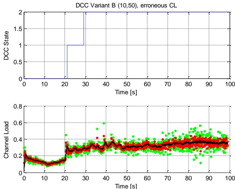
**Figure 5-15: DCC state adaptation and measured channel load of vehicle ID2 for DCC variant B with  $NDL\_TimeUp = 1s$ ,  $NDL\_TimeDown = 5s$ , 128 vehicles**
