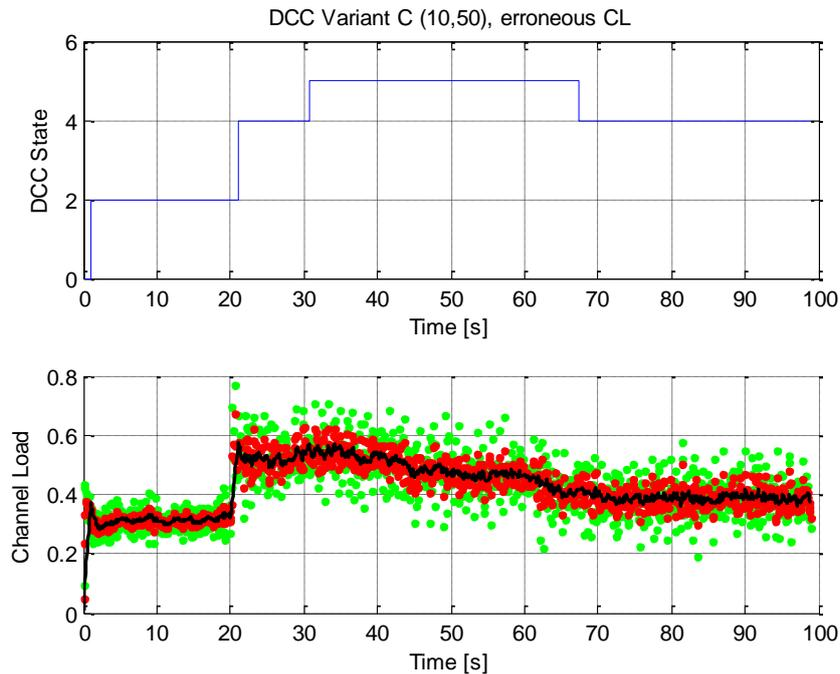
Figure 5-60: DCC state adaptation and measured channel load of vehicle ID2 for DCC variant C with  $NDL\_TimeUp = 1s$ ,  $NDL\_TimeDown = 5s$ , 256 vehicles
