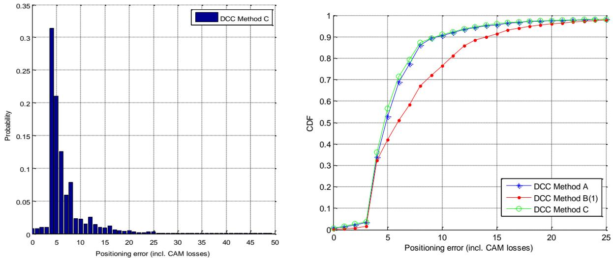
**Figure 5-39: Probability of position error for DCC variant C (left) and cumulative distribution function of selected DCC variants based on received CAM packets, 128 vehicles**
