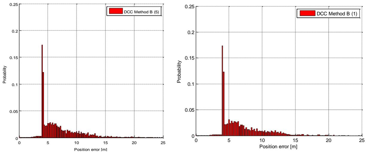
**Figure 5-34: Probability of position error for DCC variant B with a CAM queue length of 5 (left) and 1 (right) based on CAM packet transmissions, 128 vehicles**
