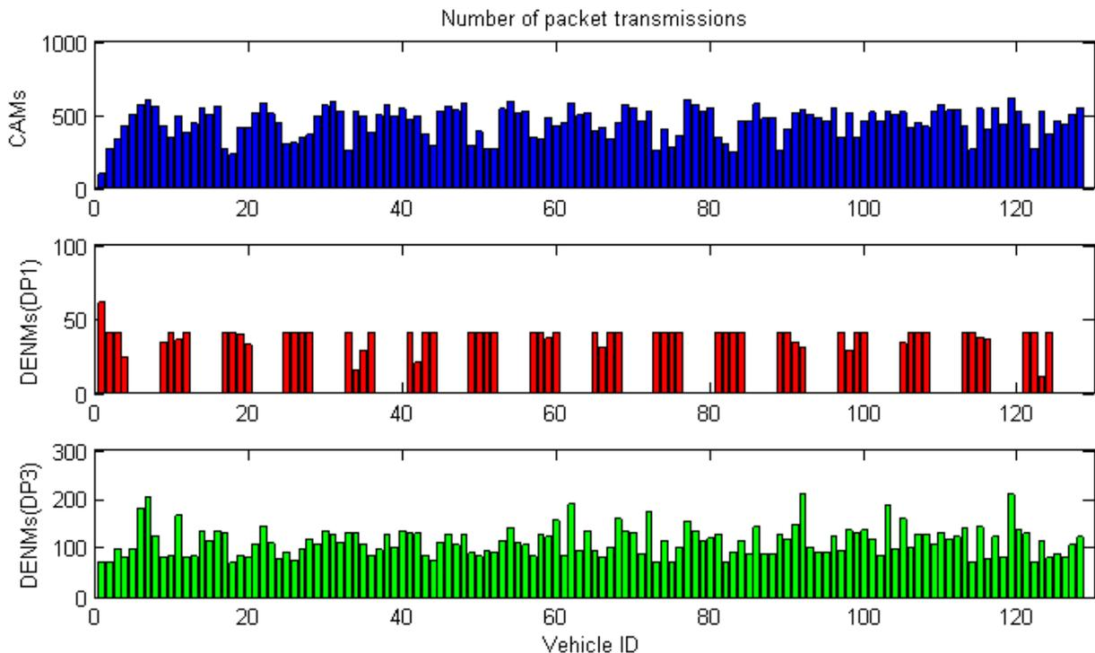
Figure 5-24: Number of transmitted packets as a function of priority, modified DCC variant A, 128 vehicles
