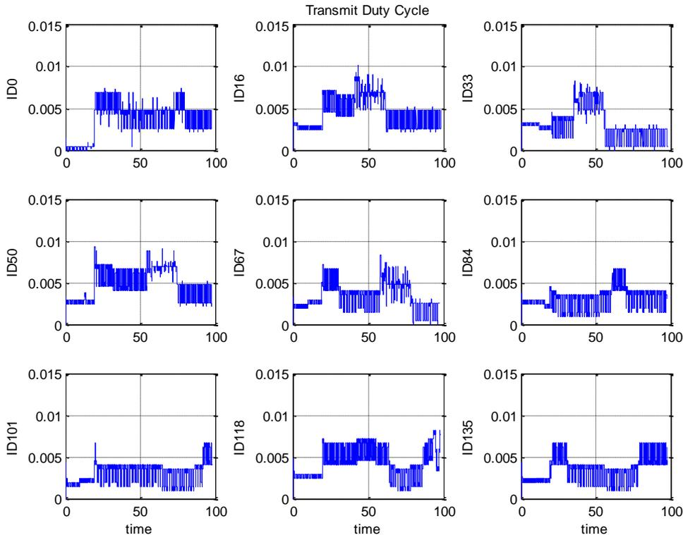
Figure 5-63: Duty cycle for 9 selected vehicles, DCC variant C, 256 vehicles
