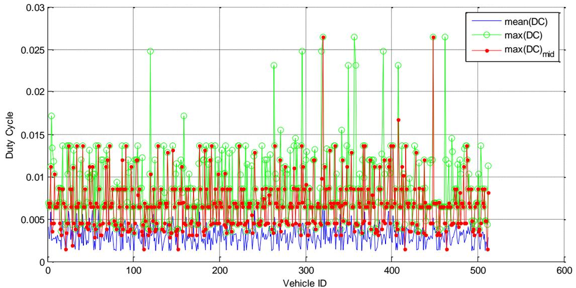
**Figure 5-83: Mean and maximum duty cycle, DCC variant B, 512 vehicles**
