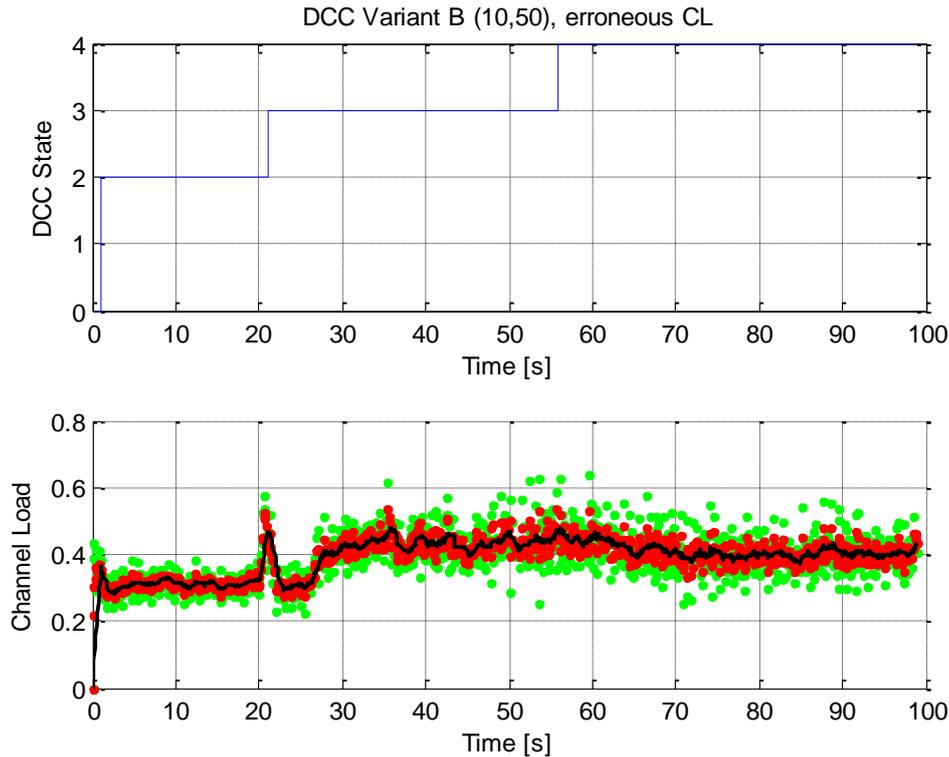
**Figure 5-49: DCC state adaptation and measured channel load of vehicle ID2 for DCC variant B with  $NDL\_TimeUp = 1s$ ,  $NDL\_TimeDown = 5s$ , 256 vehicles**
