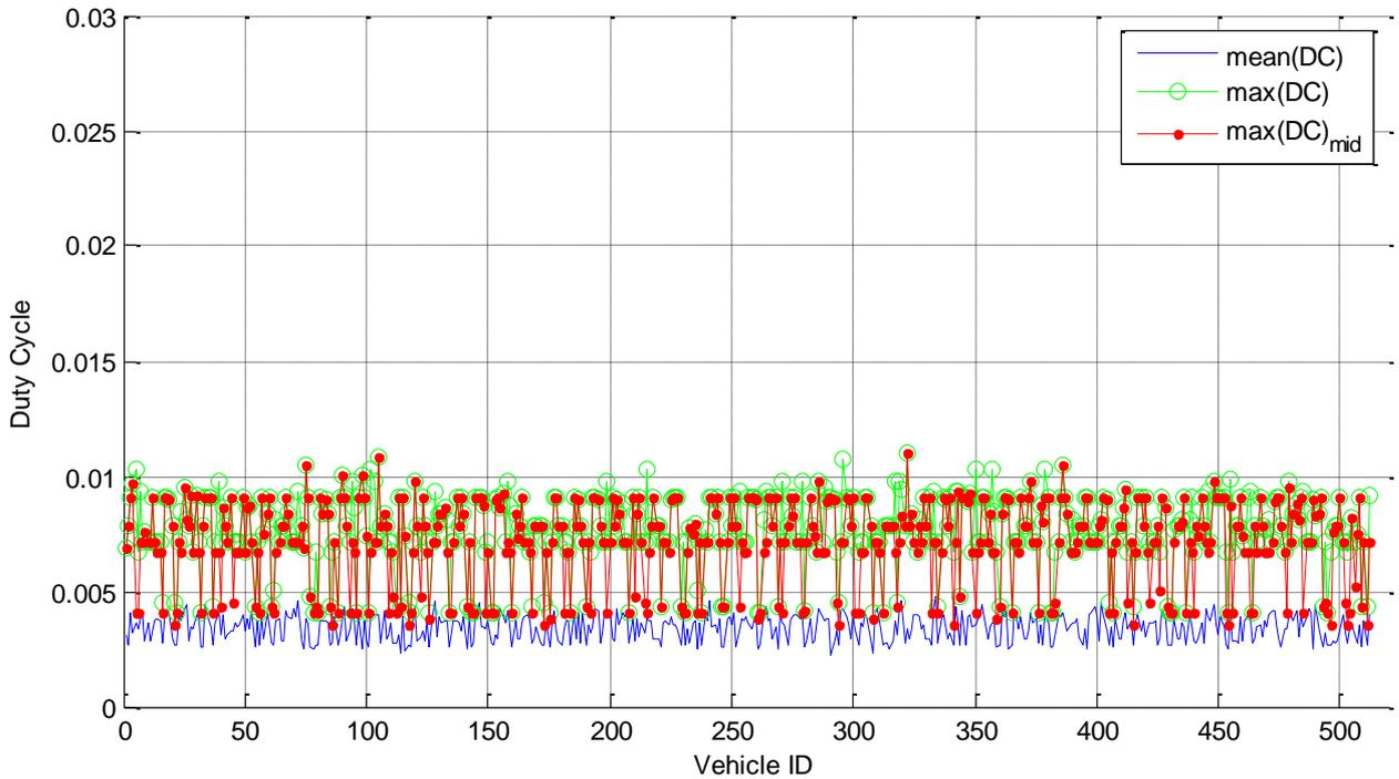
Figure 5-93: Mean and maximum duty cycle, DCC variant C, 512 vehicles
