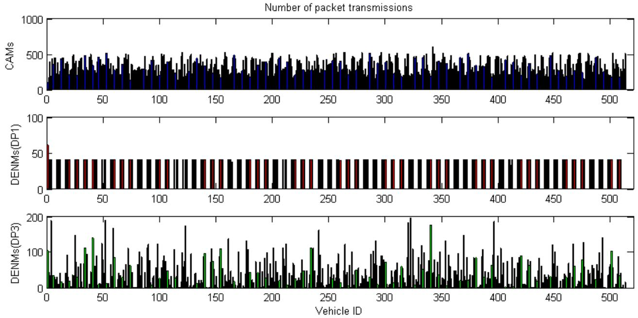
Figure 5-80: Number of transmitted packets as a function of priority, DCC variant B, 512 vehicles
