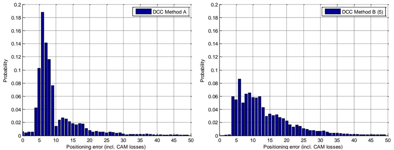
**Figure 5-97: Probability of position error for DCC variant A (left) and DCC variant B with a CAM queue length of 5 (right) based on received CAM packets, 512 vehicles**
