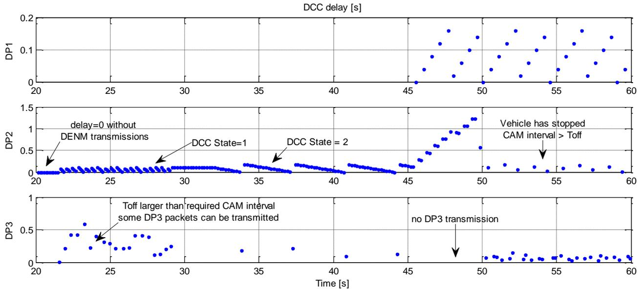
**Figure 5-16: Priority dependent DCC delay for vehicle ID2 in the highway scenario with 128 vehicles**
