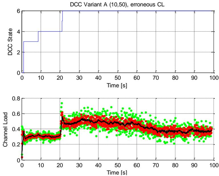
**Figure 5-43: DCC state adaptation and measured channel load of vehicle ID2 for DCC variant A with  $NDL\_TimeUp = 1s$ ,  $NDL\_TimeDown = 5s$ , 256 vehicles**
