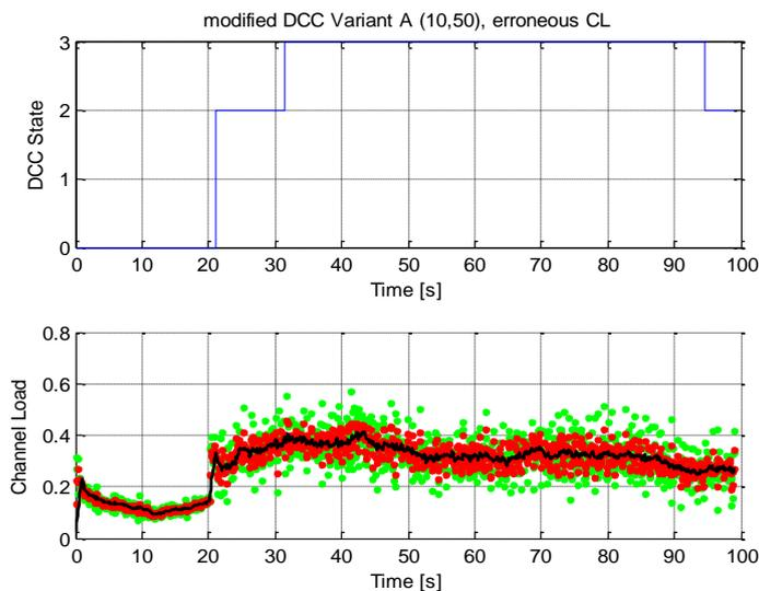
**Figure 5-23: DCC state adaptation and measured channel load of vehicle ID2 for modified DCC variant A with  $NDL\_TimeUp = 1s$ ,  $NDL\_TimeDown = 5s$ , 128 vehicles**
