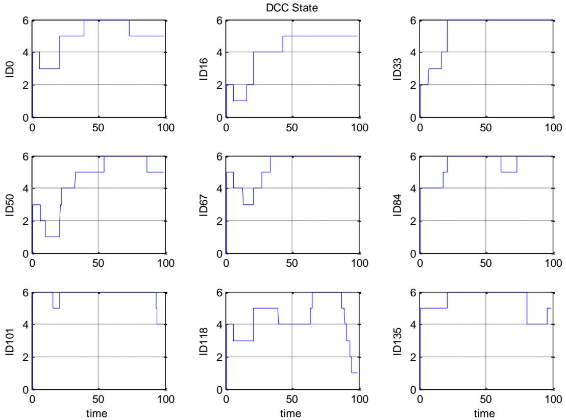
Figure 5-46: DCC state for 9 selected vehicles, DCC variant A, 256 vehicles
