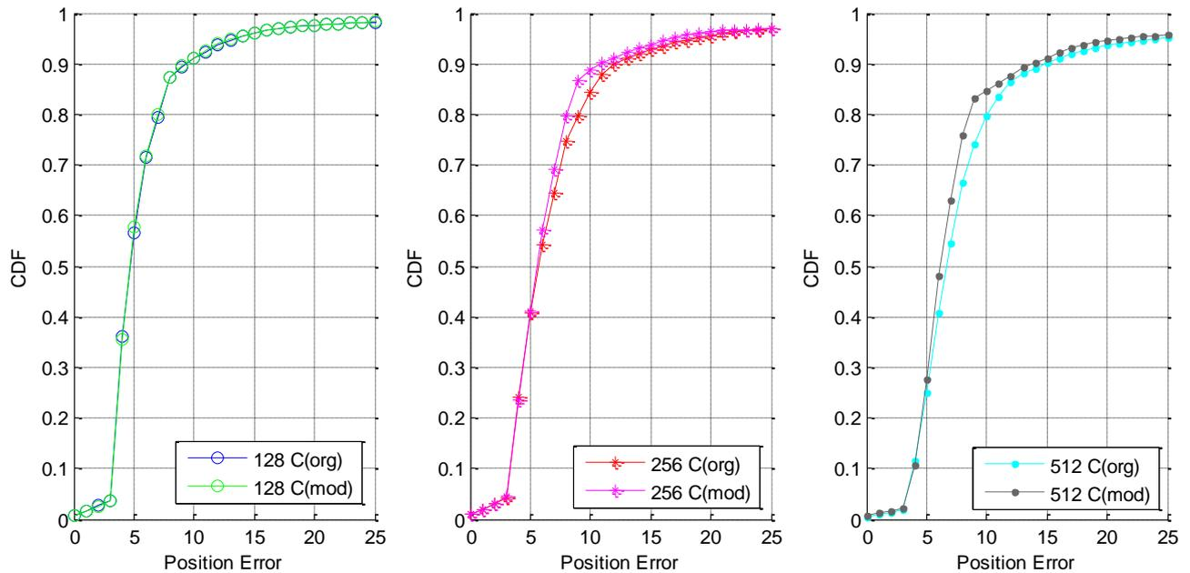
**Figure 6-1: CDF of the position error based on CAM receptions for the original and the modified DCC variant C and 128, 256 and 512 vehicles**
