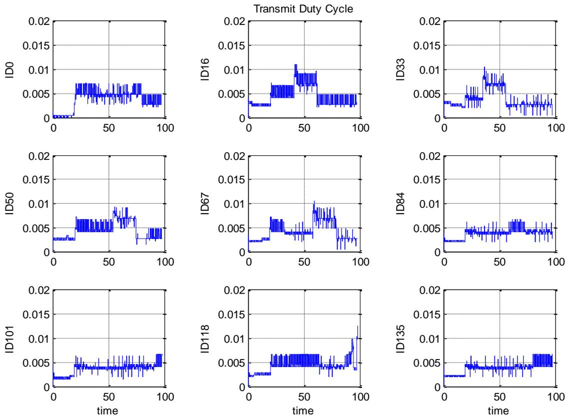
Figure 5-47: Duty cycle for 9 selected vehicles, DCC variant A, 256 vehicles
