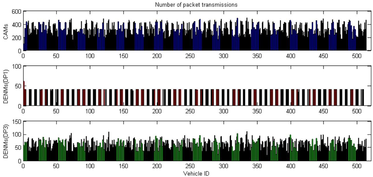
Figure 5-90: Number of transmitted packets as a function of priority, DCC variant C, 512 vehicles
